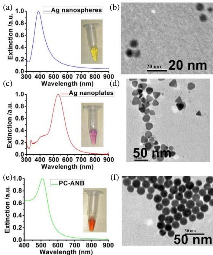
**Figure 2.** (a), (c), (e) Are the extinction spectra of Ag nanospheres, Ag nanoplates and PC-ANB, and the insets are the pictures of their corresponding solution, respectively. (b), (d), (f) Are the corresponding TEM images of the Ag nanospheres, Ag nanoplates and PC-ANB. The scale bars are 20 nm, 50 nm, 50 nm, respectively.
