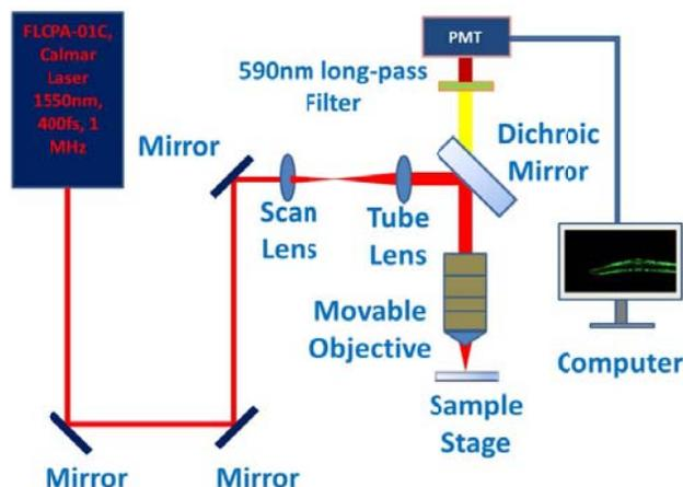
**Figure 1.** The optical set-up of 3PL imaging microscope.
