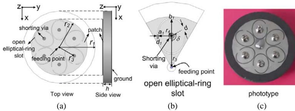
**Figure 3.** Geometry and photograph of the proposed antenna with the sizes of  $r_1 = 30$  mm,  $r_2 = 23.4$  mm,  $r_3 = 14.4$  mm,  $r_4 = 1.5$  mm,  $a_1 = 6.1$  mm,  $b_1 = 7.93$  mm,  $h = 6$  mm,  $d_1 = 3$  mm,  $d_2 = 0.4$  mm, and  $\delta = 120^\circ$ . (a) Top and side view of the proposed antenna. (b) The details of the open elliptical-ring slot. (c) Photograph of the proposed antenna.
