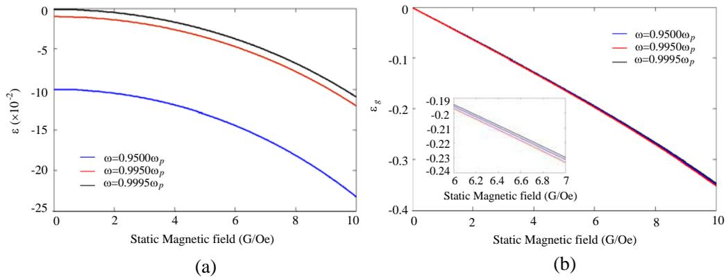
**Figure 2.** (Color online)  $\varepsilon$  and  $\varepsilon_g$  of magnetized plasma versus magnetic field at  $\omega = 0.9995\omega_p$ ,  $\omega = 0.9975\omega_p$ , and  $\omega = 0.9950\omega_p$ . The variation of  $\varepsilon_g$  is greater than  $\varepsilon$  during the magnetization process which indicates that at frequencies near the plasma frequency,  $\varepsilon_g$  will play the dominant role to determine the electromagnetic properties of the magnetized plasma.
