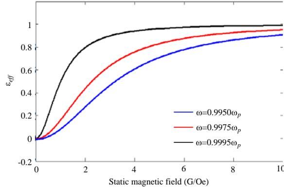
**Figure 3.** (Color online) Magneto-permittivity of the magnetized plasma at  $\omega = 0.9995\omega_p$ ,  $\omega = 0.9975\omega_p$ , and  $\omega = 0.9950\omega_p$ . The effective permittivity increases during the magnetization process and becomes practically constant when the magnetization is saturated.
