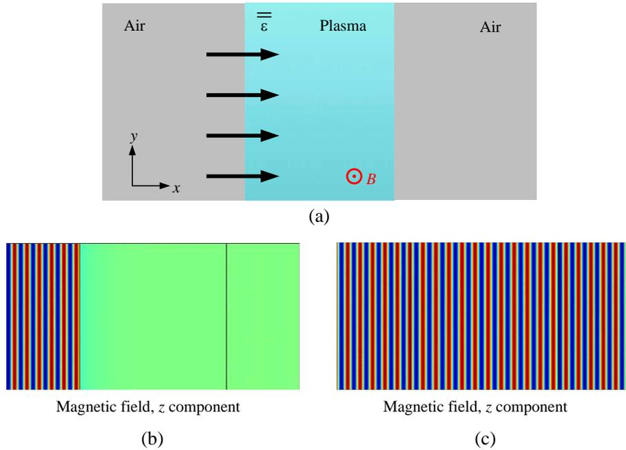
**Figure 4.** (Color online) (a) Schematic of a magnetic field switching system based on magnetized plasma. Electromagnetic wave (dark arrows) is normal incident from air to the magnetized plasma. (b)–(c) Numerical simulations of the lossless magnetized plasma at  $0.9 \times 10^8$  Hz (b) for nonmagnetized plasma and (c) for magnetized plasma with saturation magnetic field ( $\approx 10$  G).
