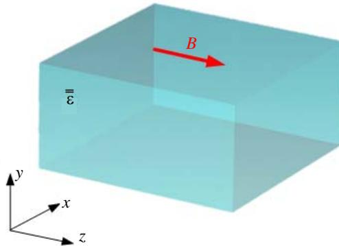
**Figure 1.** (Color online) Schematic of the bulk magnetized plasma. The red arrow represents the external magnetic field. The wave propagation is in the direction perpendicular to the magnetization direction.
