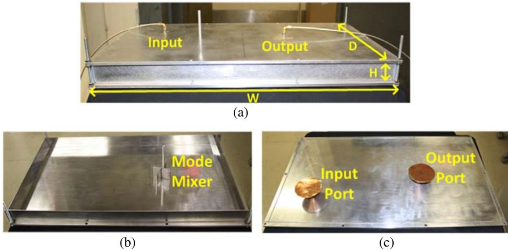
**Figure 9.** The compact reverberant cavity used in the pulse compressor experiment: (a) Overall exterior view ( $W$ ,  $H$  and  $D$  correspond to the inner dimensions), (b) cavity with the top plate off, showing the inside, and (c) the interior part of the top plate, showing the input and output ports.
