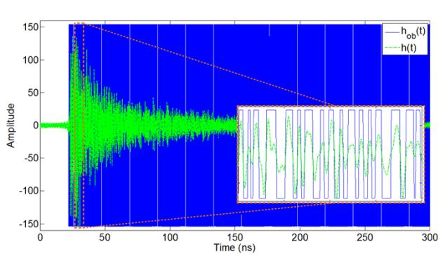
**Figure 5.** One-bit cavity impulse response,  $h_{ob}(t)$ , in comparison to the original impulse response  $h(t)$ .
