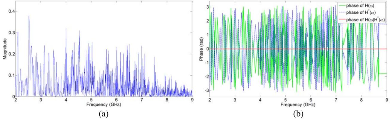
**Figure 4.** Frequency domain plot of the cavity output after TR,  $Y(\omega)$ : (a)  $|Y(\omega)|$  and (b) phase of  $|Y(\omega)|$  without  $e^{j\omega T}$  term (red) in comparison with phases of  $H(\omega)$  (green) and  $H_{ob}^*(\omega)$  (blue).
