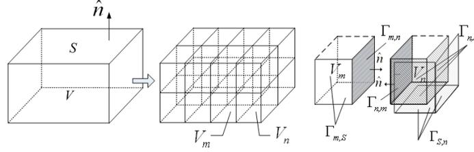
**Figure 1.** Illustration of domain decomposition method of FE-BI-MLFMA.
