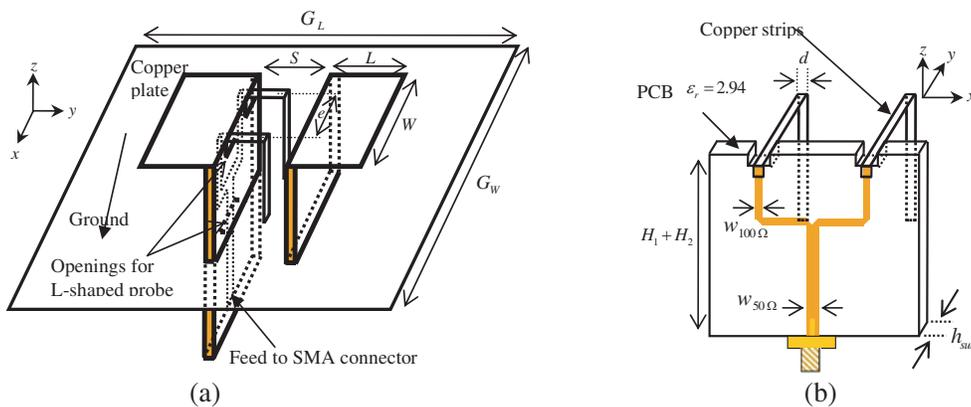
**Figure 2.** Sketch of the twin-fed configuration of the linearly polarized wideband antenna. (a) 3D sketch of the twin fed antenna. (b) Feeding details (3D).
