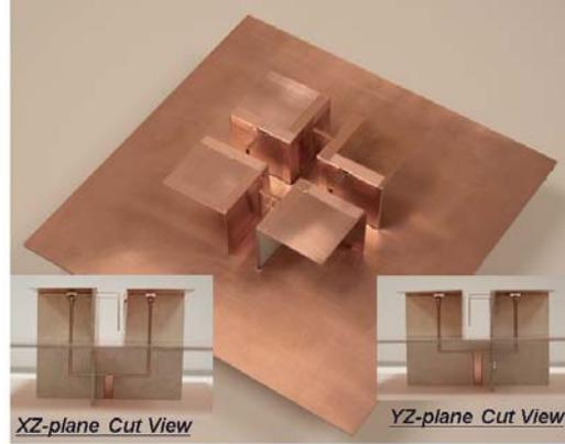
**Figure 7.** Photo of a dual-polarized wideband antenna.
