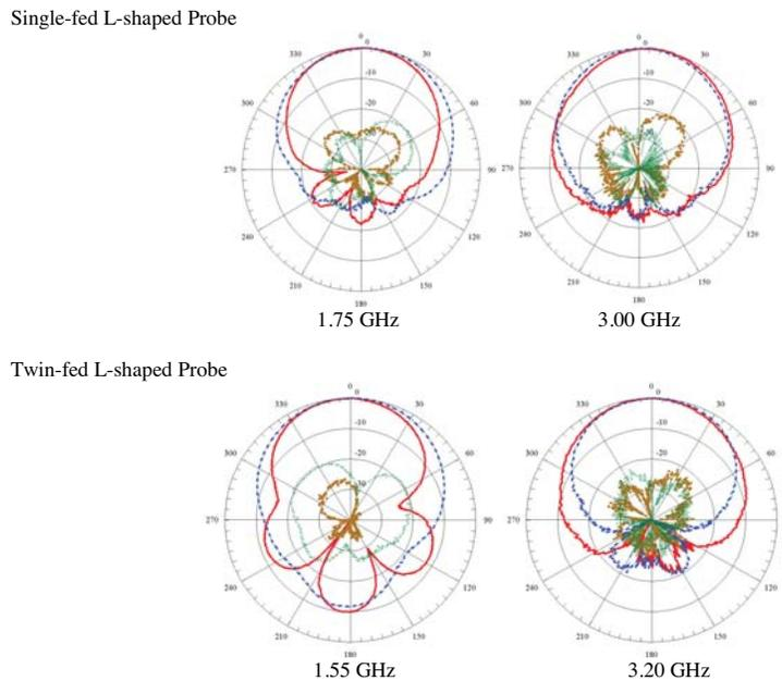
**Figure 6.** Measured radiation patterns of the antennas with single and twin L-shaped probes: Top for single L-shaped probe at 1.75, 2.50 and 3.00 GHz, and bottom for twin hook-shaped probes at 1.55, 2.50 and 3.20 GHz. Legends are the same as Fig. 5.
