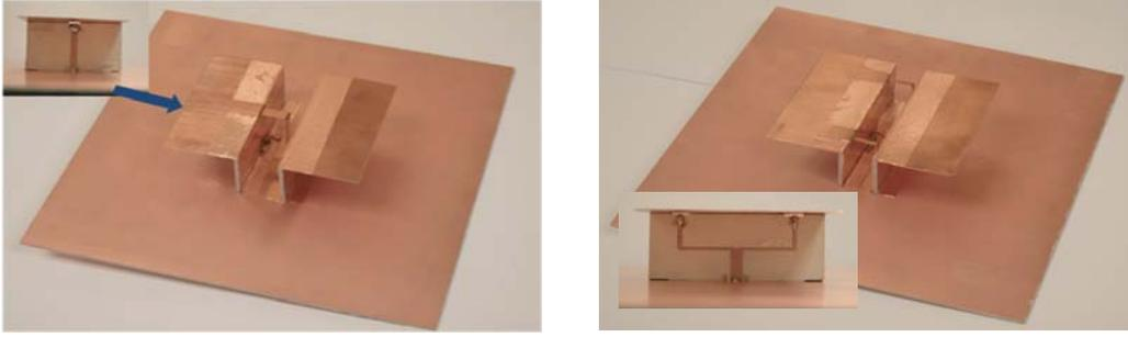
**Figure 3.** Photos for single and twin-fed L-shaped antenna.
