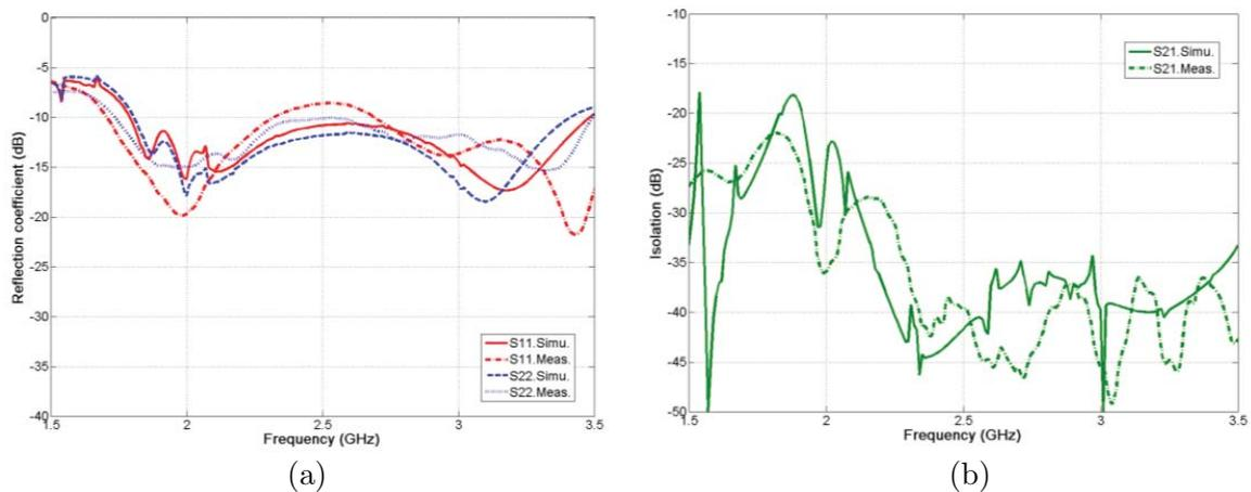
**Figure 9.** Measured and simulated isolation for a wideband dual-polarized antenna. (a) Reflection coefficients. (b) Coupling coefficients.
