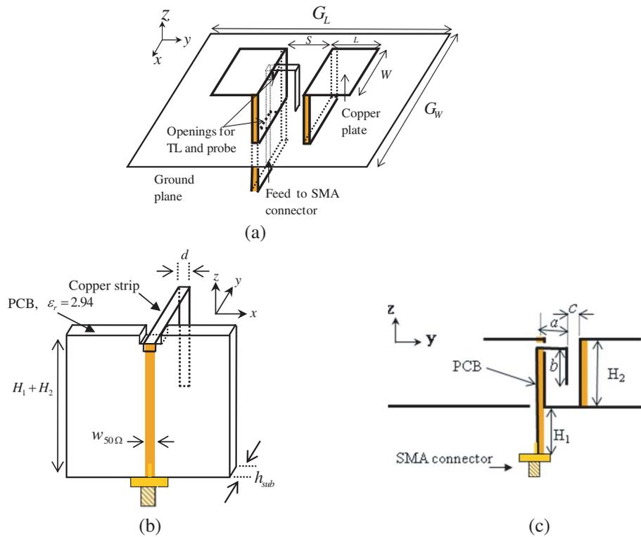
**Figure 1.** Sketch of the single-fed configuration of the linearly polarized wideband antenna. (a) 3D sketch of the single fed antenna. (b) Feeding part details (3D view). (c) Side view of the antenna.
