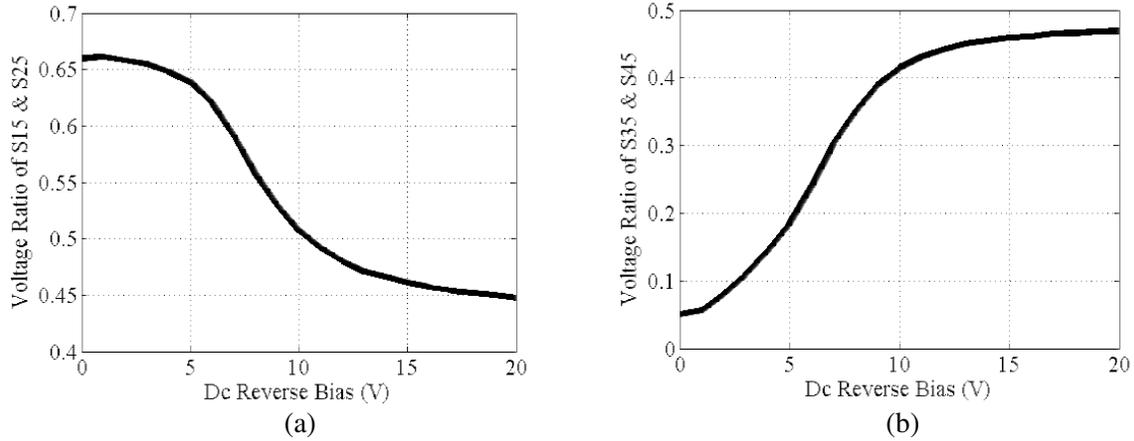
**Figure 9.** Measured voltage ratios vs. the applied DC reverse bias voltages at 5 GHz for the controllable 4-way power divider. (a) Voltage ratios of  $S_{15}$  and  $S_{25}$ . (b) Voltage ratios of  $S_{35}$  and  $S_{45}$ .
