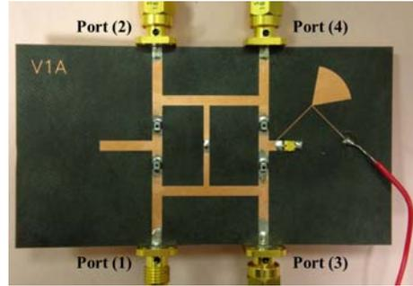
**Figure 5.** Configuration of the controllable 4-way power divider.
