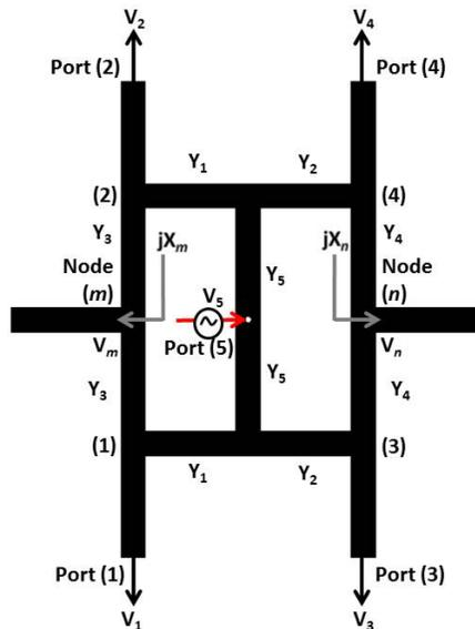
**Figure 1.** The design configuration of the proposed 5-port power dividers.
