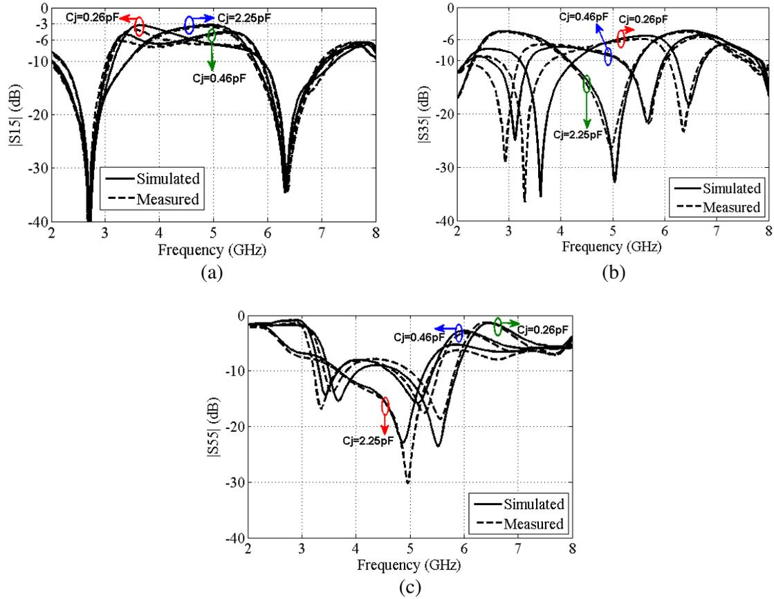
**Figure 7.** (a) Measurement vs. simulation results of  $|S_{15}|$ . (b) Measurement vs. simulation results of  $|S_{35}|$ . (c) Measurement vs. simulation results of  $|S_{55}|$ .
