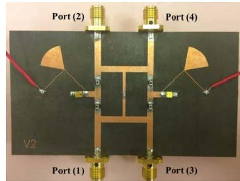
**Figure 2.** Configuration of the switchable 2-way power divider.
