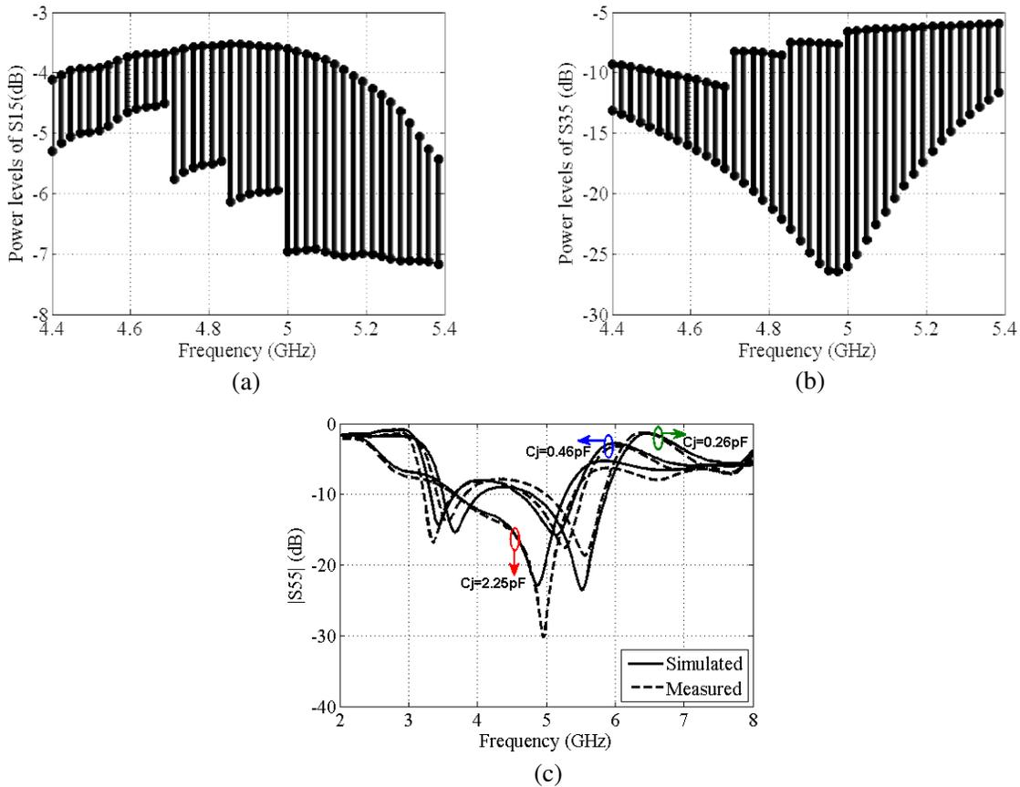
**Figure 8.** Available power levels while adjusting  $C_j$  value within the acceptable capacitance ranges. (a)  $S_{15}$ . (b)  $S_{35}$ . (c)  $S_{55}$ .
