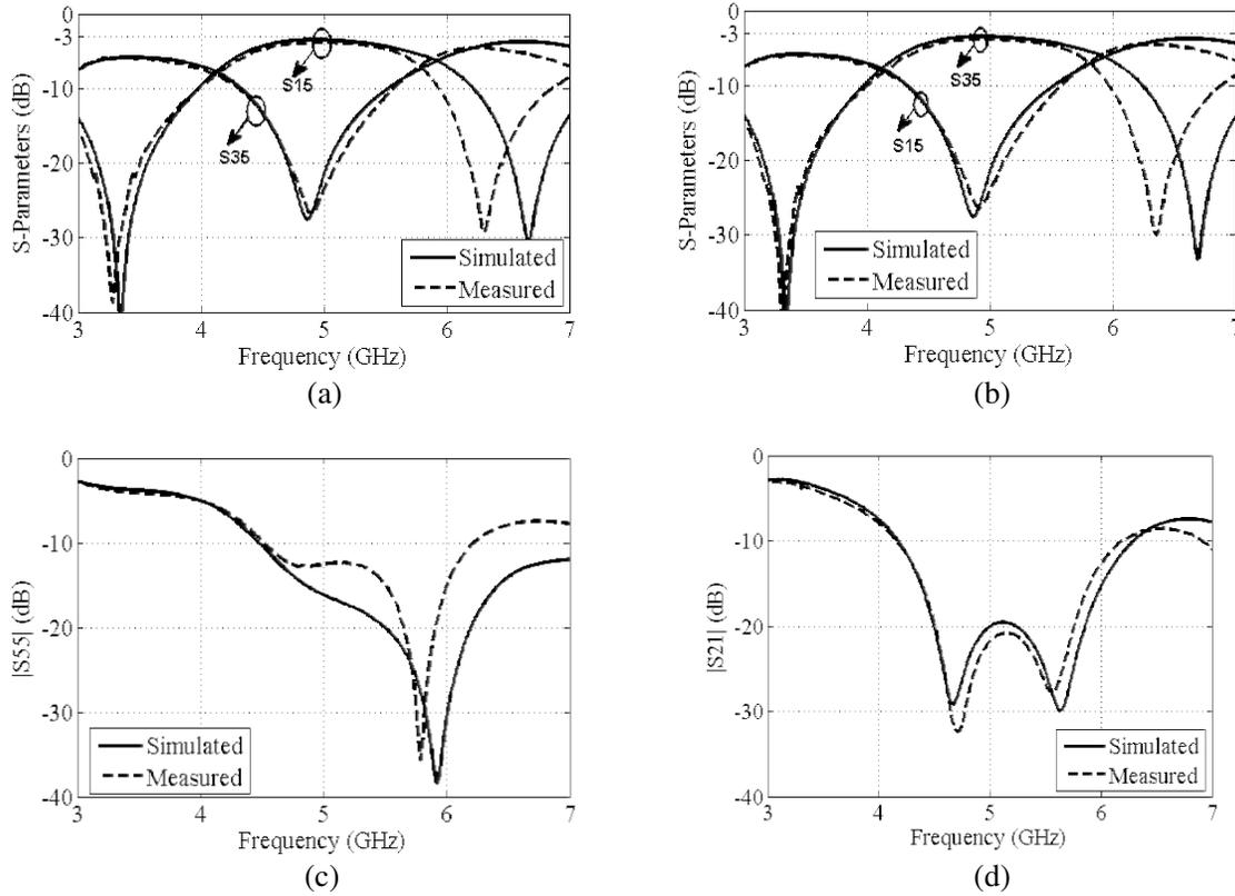
**Figure 4.** (a) Measurement vs. simulation results for  $|S_{15}|$  and  $|S_{35}|$  (State A). (b) Measurement vs. simulation results for  $|S_{15}|$  and  $|S_{35}|$  (State B). (c) Measurement vs. simulation results for  $|S_{55}|$  (identical for both states). (d) Measurement vs. simulation results for  $|S_{21}|$  (State A).
