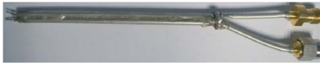
Figure 6. Differential probe used to characterize the antennas.
