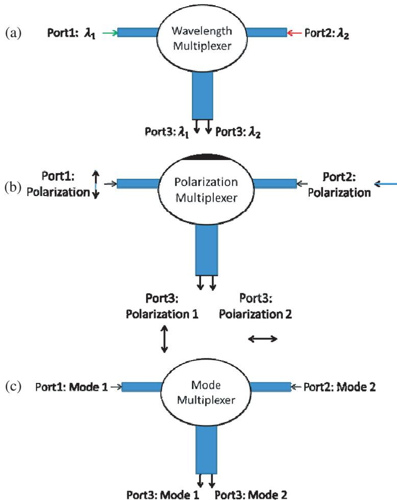
**Figure 5.** Perfect power combiners for waves of (a) different wavelengths; (b) different polarizations; and (c) different modes.
