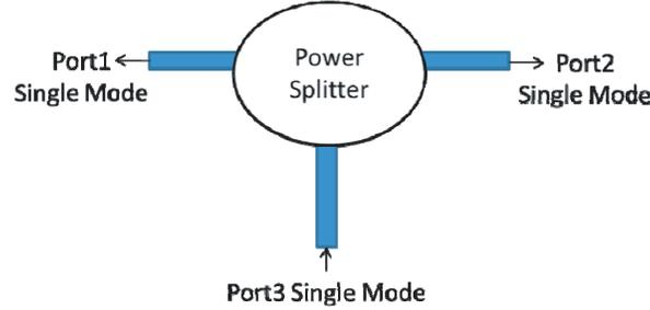
**Figure 1.** A schematic diagram for a power splitter.
