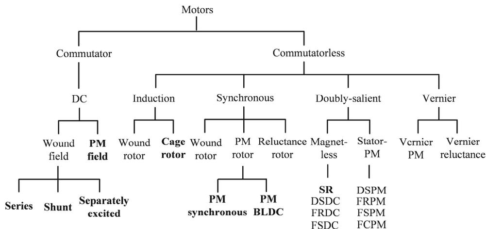
Figure 2. Classification of electric motors for electric propulsion.
