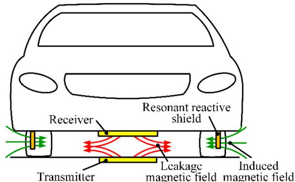
**Figure 5.** Resonant reactive shielding for wireless charging.
