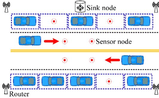
**Figure 7.** Vehicle static and dynamic detections using magnetic sensors.
