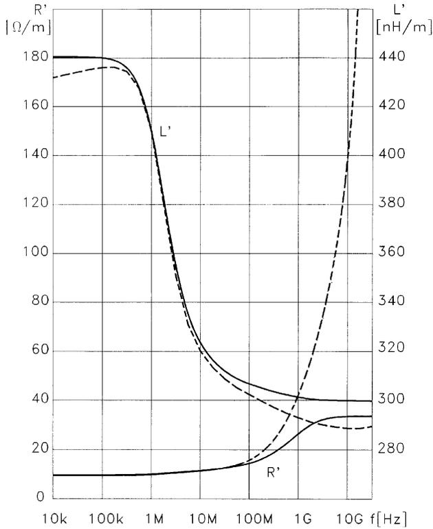
**Figure 5.** Resistance per unit length ( $R'$ ) and inductance per unit length ( $L'$ ) of the microstrip line of Figure 4, versus frequency ( $f$ ), computed using the volume-current formulation (—) and the surface-current formulation (---).
