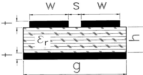
**Figure 6.** Sketch of two coupled microstrip line.
