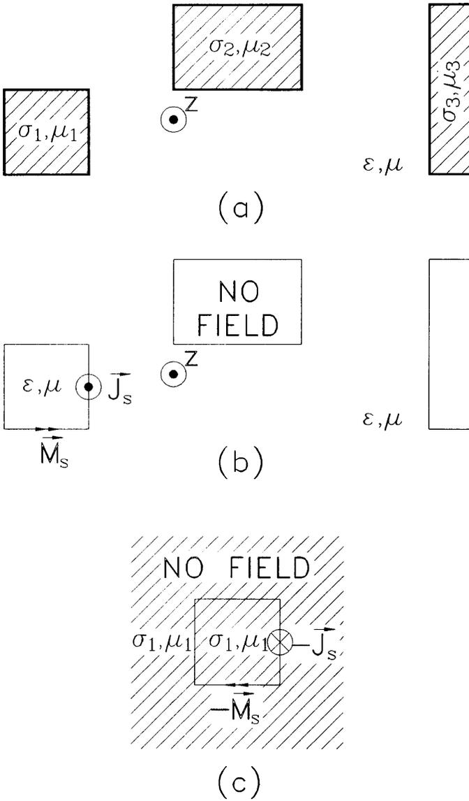
**Figure 2.** (a) Cross section of the array of Figure 1, and the equivalent systems for (b) the exterior region, and (c) interior region of conductor #1.
