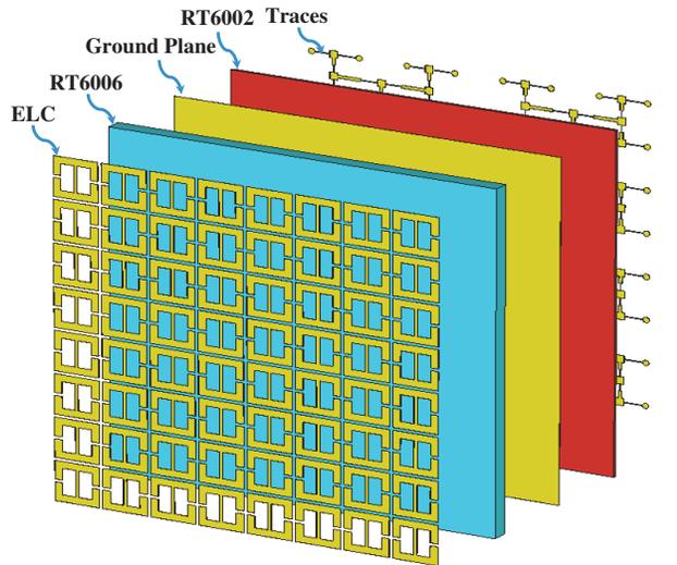
**Figure 3.** Schematic of the metasurface shown as an exploded view including the ELC resonators, Rogers RT6006 material as the first substrate, ground plane (copper), Rogers RT6002 as the second substrate, and the transmission line traces.
