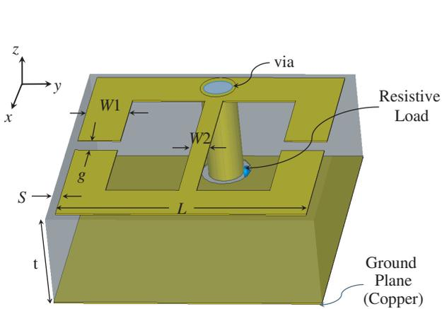
**Figure 1.** A schematic of the ELC unit cell. The incident field is a plane wave incident in the  $-z$  direction and  $E$ -polarized in the  $x$  direction.
