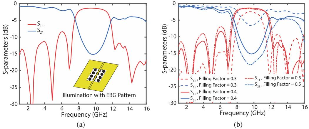
**Figure 5.** (a) Simulated  $S$ -parameters of the prototype BSF with an EBG photo-induced pattern (as illustrated in Fig. 3(b)). (b) Simulated  $S$ -parameters of the prototype with three different EBG photo-patterns with fixed period of 5.7 mm but different filling factor (0.3, 0.4, and 0.5, respectively).
