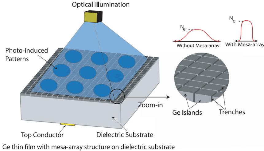
**Figure 7.** Illustration of a Ge-based mesa-array structure on a dielectric substrate. The mesa-array structure consists of a matrix of Ge islands. Each island is electrically isolated to prevent lateral diffusion, and the dimensions are much smaller than either the wavelength or the carrier diffusion length.
