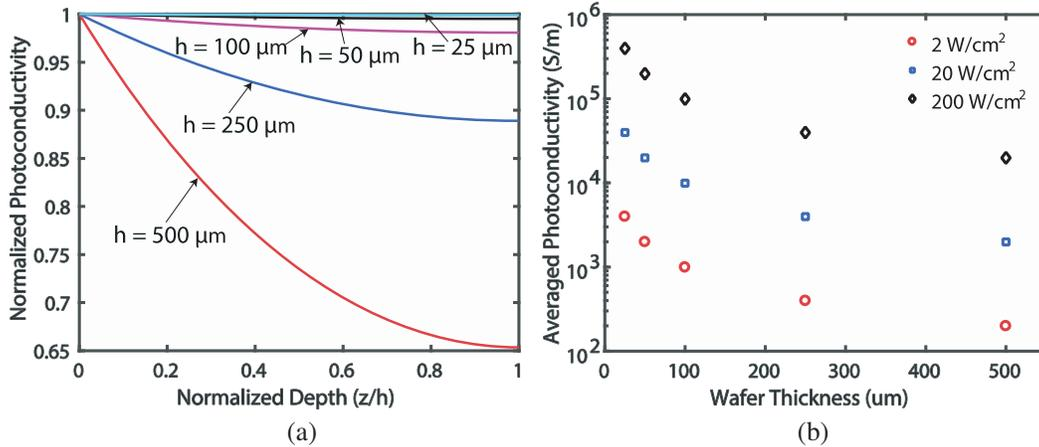
**Figure 2.** (a) Normalized photoconductivity as a function of depth into Ge for different wafer thicknesses (i.e., 25 μm, 50 μm, 100 μm, 250 μm and 500 μm, respectively) illuminated by continuous 550 nm light. (b) Spatially averaged photoconductivity in Ge as a function of wafer thickness and light intensity (i.e., 2 W/cm<sup>2</sup>, 20 W/cm<sup>2</sup>, and 200 W/cm<sup>2</sup>, respectively).
