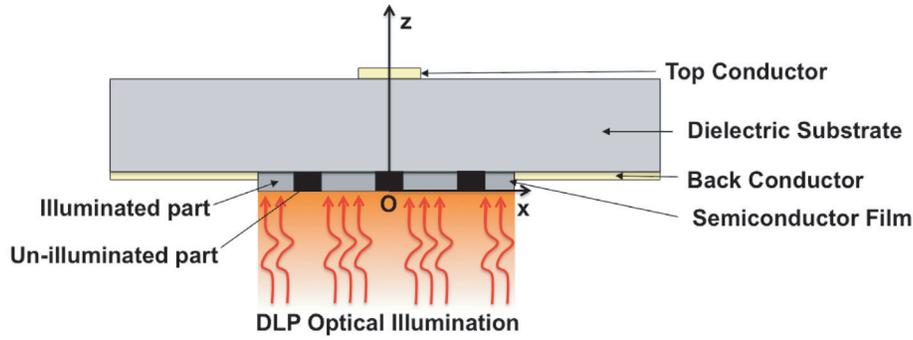
**Figure 1.** Cross-sectional view of the proposed structure for implementing optically-controlled tunable and reconfigurable uniplanar EBG component in a microstrip line configuration. Virtual EBG patterns are projected onto the semiconductor film using a DLP projector to form uniplanar EBG configuration with tunable properties.
