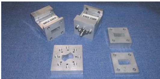
Figure 5. Picture of the fabricated twist along with coaxial-to-waveguide transitions and delay lines acting as \lambda_g/4 standards for the TRL calibration.
