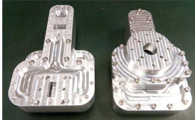
**Figure 9.** OMT platelet prototypes.
