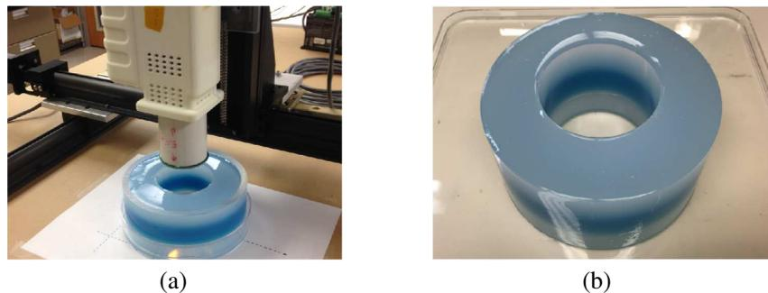
**Figure 2.** (a) Agarose phantom resting on the positioning stage, just beneath a stub-mounted 5.0 cm diameter coil, which is relocated by the 3-axis controller affixed to the same stage; (b) Close up view of the annular phantom and its central cavity — the blue, 2.0 cm thick embedded annular inclusion is doped with NaCl, elevating its “uniform” conductivity above surrounding agarose.
