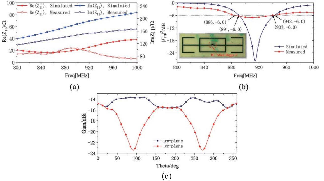
**Figure 3.** (a) The simulated and measured input impedance of the simple design. (b) The simulated and measured  $|\Gamma_m|^2$  of the simple design. (c) The simulated curves of the gain for the simple design.
