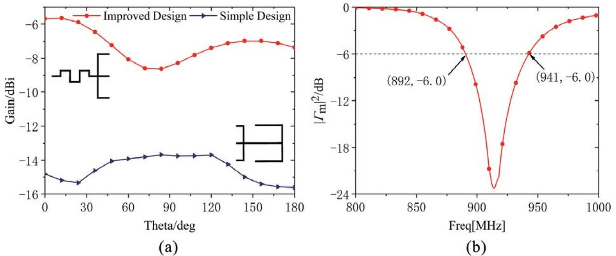
**Figure 5.** (a) The gains for the simple design and the improved design in  $xz$ -plane. (b) Curves of  $|\Gamma_m|^2$  for the improved design.
