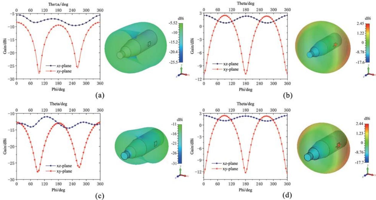
**Figure 10.** The gain and radiation pattern for the antenna with a three-loop matching structure at 915 MHz. (a) on a plastic bottle filled with water; (b) on an empty plastic bottle; (c) on a glass bottle filled with water; (d) on an empty glass bottle.
