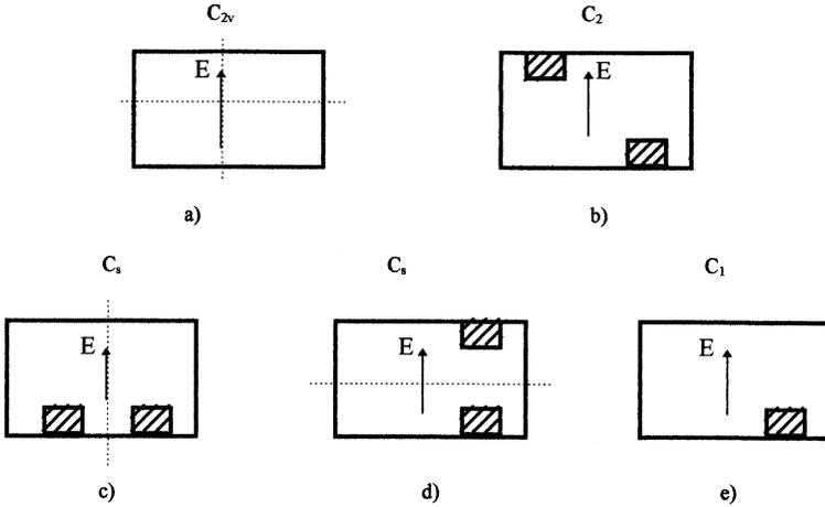
**Figure 1.** Cross-sections of rectangular waveguides with different symmetries.
