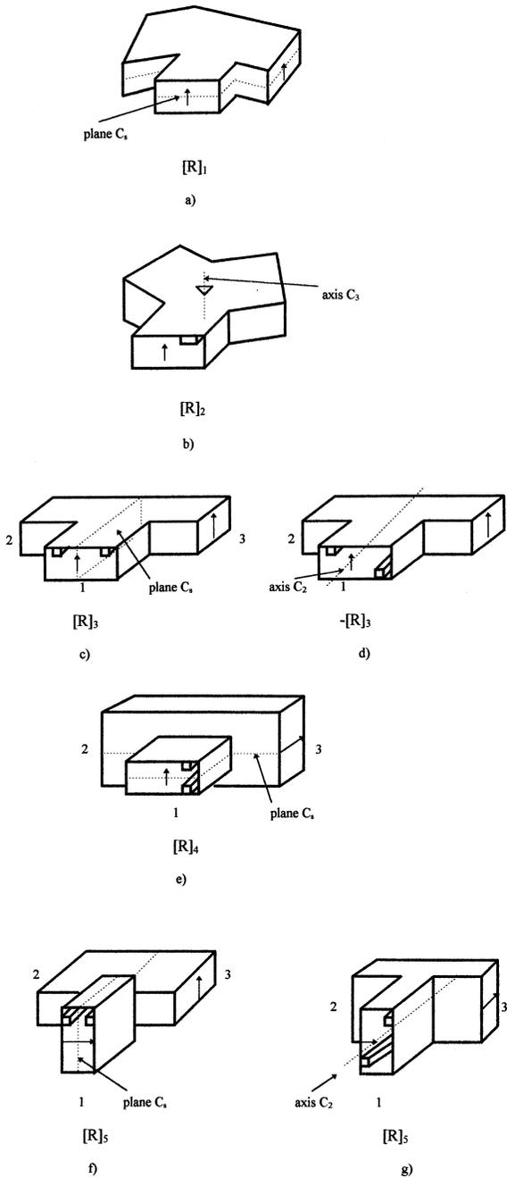
Figure 3. Examples of three-ports with different symmetries.
