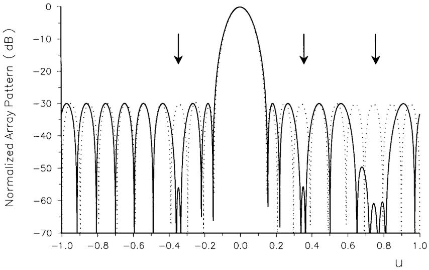
**Figure 1.** Simulated antenna array pattern: solid, perturbed pattern with three wide sectors imposed around  $u_m = -0.35, 0.35,$  and  $0.75$  for  $B = 5\%$ ,  $5\%$ , and  $10\%$ , respectively; dotted, initial 30-dB Chebyshev pattern,  $2N = 20$ ,  $d_0 = \lambda/2$ .
