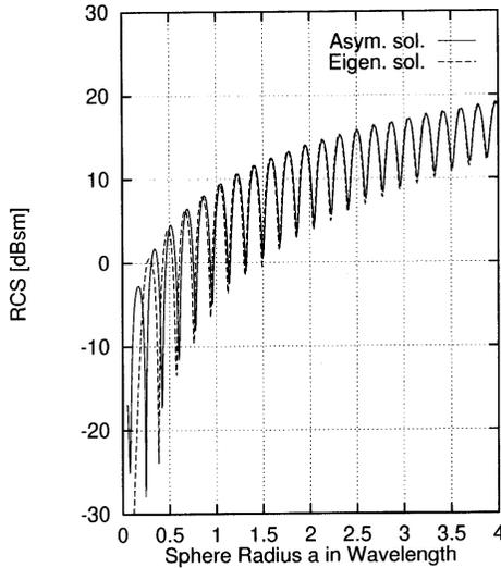
**Figure 2.** RCS from a coated sphere with the coating material  $\epsilon_r = (2.5, -0.2)$  and  $\mu_r = (1.6, -0.1)$  and the thickness of coating  $d = 0.05\lambda_0$ .
