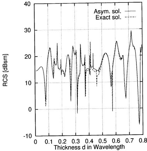
**Figure 9.** RCS from a coated sphere with  $\epsilon_r = (2.56, 0.)$ ,  $\mu_r = (1., 0.)$  and  $a = 3\lambda_o$ . It is found that as the thickness of coating is increased, the groups of resonances are occur.
