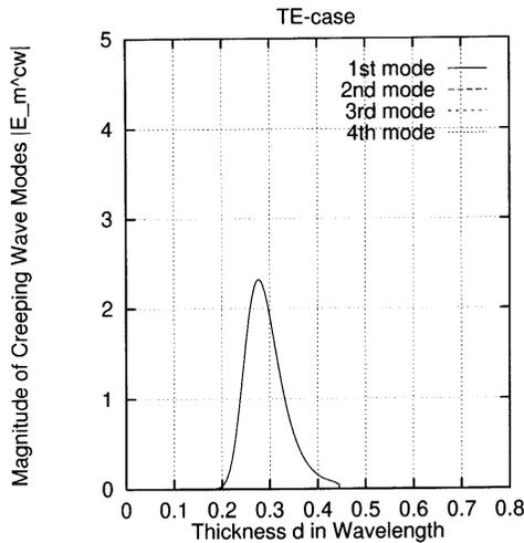
**Figure 8.** The magnitude of creeping wave modes from the attenuation constant (Fig. 5) and the diffraction coefficient (Fig. 6): TE-case. The first mode of the creeping wave is very significant when  $d = 0.28\lambda_o$  and the other modes are negligible when  $d = 0. \sim 0.8\lambda_o$ .
