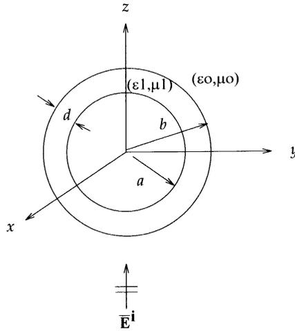
Figure 1. Geometry of the coated sphere.
