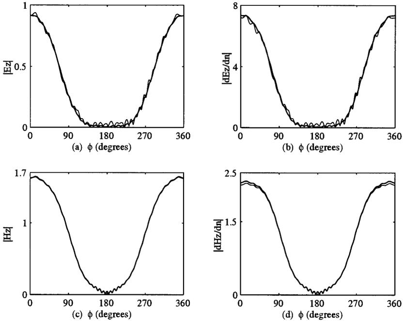
**Figure 4.** Distributions of fields and their normal derivatives on  $\Gamma$  for the conducting cylinder coated with lossy material ( $\mu_r = 1$  and  $\epsilon_r = 4 - 4i$ ) obtained by using the first method. The thicker line: the analytical solution; the thin line: the WTM solution. (a) and (b) for TM wave incidence ( $\tau/m = 1E - 8$ ), and (c) and (d) for TE wave incidence ( $\tau/m = 1E - 7$ ).
