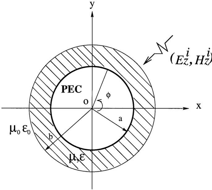
**Figure 2.** Scattering from a coated conducting cylinder.
