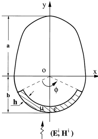
**Figure 8.** The geometry of the second problem under analysis.  $a = \frac{40.63}{\pi}\lambda$ ,  $b = \frac{20}{\pi}\lambda$ ,  $\epsilon_r = 2.5(1 - 0.01i)$ ,  $\mu_r = 1.0$ ,  $f = 5GHz$ ,  $h = 0.3\lambda$ ,  $\phi = \pi.2$ ,  $\phi_i = -\pi/2$ , under TM plane wave incidence.
