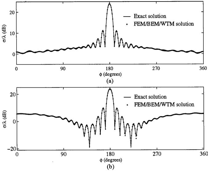
**Figure 7.** RCS for the conducting cylinder coated with lossy material ( $\mu_r = 1$  and  $\epsilon_r = 4 - 4i$ ) by using the second method. (a) under TM wave incidence ( $\tau/m = 1E - 5.5$ ); (b) under TE wave incidence ( $\tau/m = 1E - 5.5$ ).
