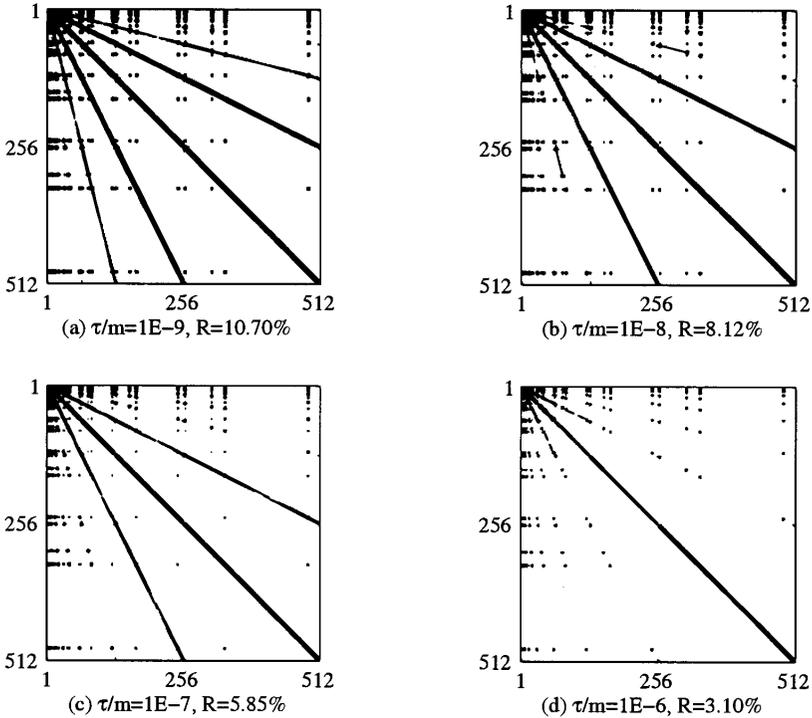
**Figure 9.** The remaining nonzero elements of  $A'$  for the second problem under analysis by using the second method after setting to zero each element whose magnitude is smaller than a selected threshold  $\tau$  for the TM case.
