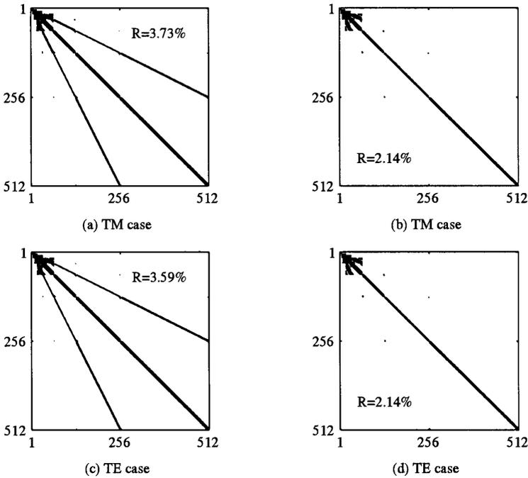
**Figure 6.** The remaining nonzero elements of  $A'$  by using the second method after setting to zero each element whose magnitude is smaller than a selected threshold  $\tau$ . (a) and (c)  $\tau/m = 10^{-6}$ . (b) and (d)  $\tau/m = 10^{-5.5}$ .
