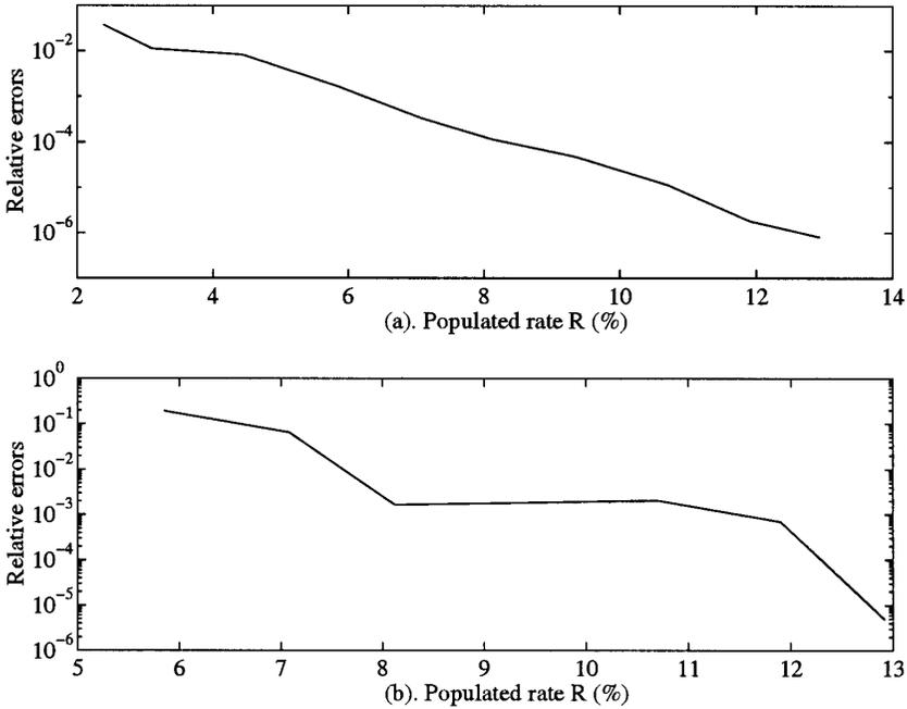
**Figure 10.** The relative error of solutions by the NS-NCSW transforms versus the populated rate  $R$  for the second problem under analysis. Reference solution is solved from the relevant dense matrix equation. (a). for  $u$  (b). for  $\Psi$ .
