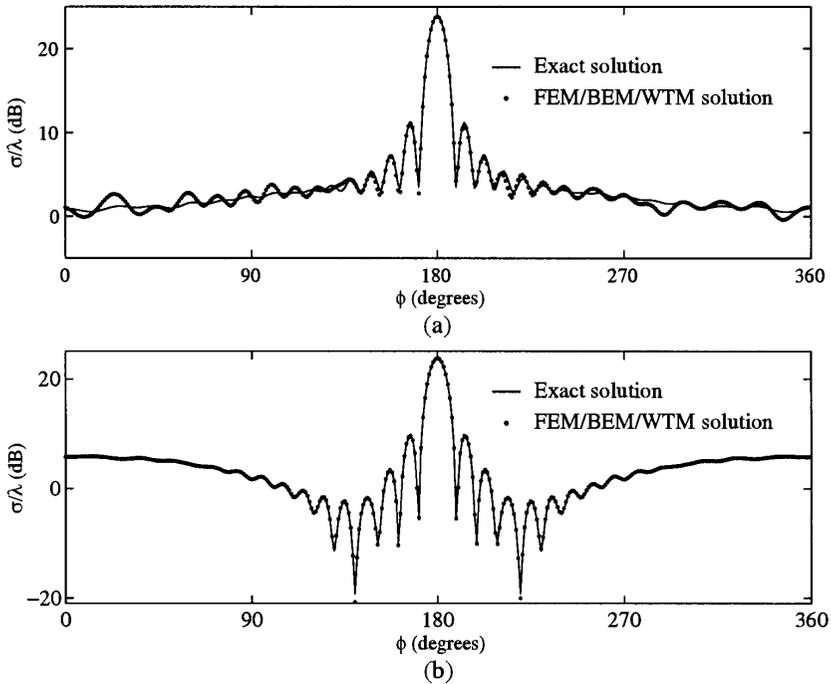
**Figure 5.** RCS for the conducting cylinder coated with lossy material ( $\mu_r = 1$  and  $\epsilon_r = 4 - 4i$ ) obtained by using the first method. (a) under TM wave incidence ( $\tau/m = 1E - 8$ ); (b) under TE wave incidence ( $\tau/m = 1E - 7$ ).
