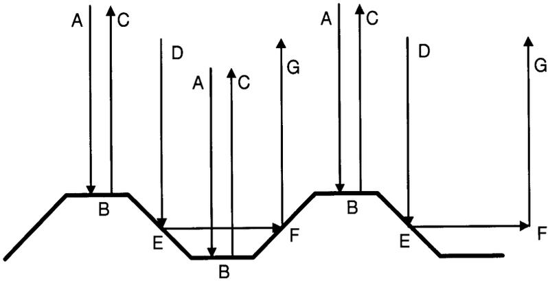
**Figure 1.** Specular mirroring mechanisms expected in the presence of corrugated and cylinder-lined surfaces.  $A \rightarrow B \rightarrow C$  is a (simple reflection process, but  $D \rightarrow E \rightarrow F \rightarrow G$  is a retrodirective process.
