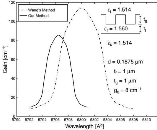
**Figure 8.** Gain (imaginary part of the propagation constant) for the structure shown in the insert calculated by our method (solid line) and by Wang's model (dashed line).  $d$  and  $g_0$  are period of the grating and the gain of the active layer ( $\epsilon_f = 1.560$ ), respectively.
