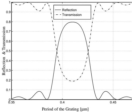
**Figure 6.** Reflection and transmission characteristics of the filter illustrated in Fig. 5 versus the grating period for 20 periods.
