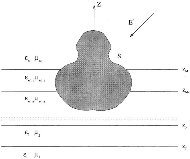
**Figure 1.** A body of revolution in layered medium.
