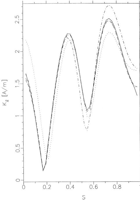
**Figure 5.** Magnitude of  $K_\ell$  on a metallic sphere present in the upper space with the parameters:  $\epsilon_1 = 10.0$ ,  $\epsilon_2 = 1.0$ ,  $\theta^i = 0.0^\circ$ ,  $k_2a = 2.744$  and  $d = 0.2\lambda_o$ . EFIE: ....., MFIE: - · - ·, CFIE: —, CFT: - - - - , CHIEF: - - - - .
