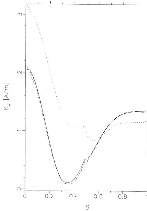
**Figure 11.** Magnitude of  $K_\varphi$  on a half-buried metallic sphere with the parameters:  $\epsilon_1 = 10.0$ ,  $\epsilon_2 = 1.0$ ,  $\theta^i = 0.0^\circ$ ,  $k_o a = 1.035$ . EFIE: ....., MFIE: —, CFT: - · · ·, CHIEF: - - - .
