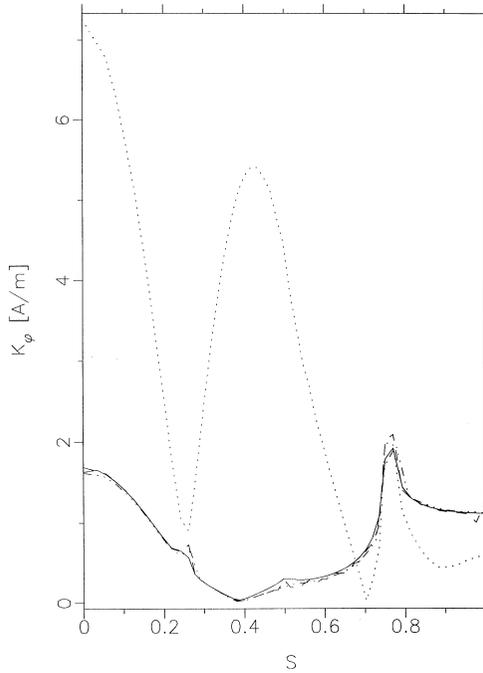
**Figure 16.** Magnitude of  $K_\phi$  on a half-buried metallic pillbox with the parameters:  $\epsilon_1 = 10.0$ ,  $\epsilon_2 = 1.0$ ,  $\theta^i = 0.0^\circ$ ,  $L/a = 2.0$  and  $k_o a = 0.9147$ . EFIE: ....., MFIE: —, CFT: - · · ·, CHIEF: - - - .
