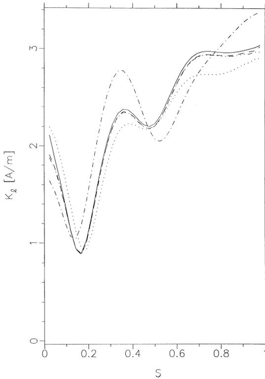
**Figure 7.** Magnitude of  $K_\ell$  on a metallic sphere present in the lower space with the parameters:  $\epsilon_1 = 10.0$ ,  $\epsilon_2 = 1.0$ ,  $\theta^i = 0.0^\circ$ ,  $k_1 a = 2.744$  and  $d = -0.4\lambda_o$ . EFIE: ....., MFIE: - · - ·, CFIE: —, CFT: - · · ·, CHIEF: - - - .
