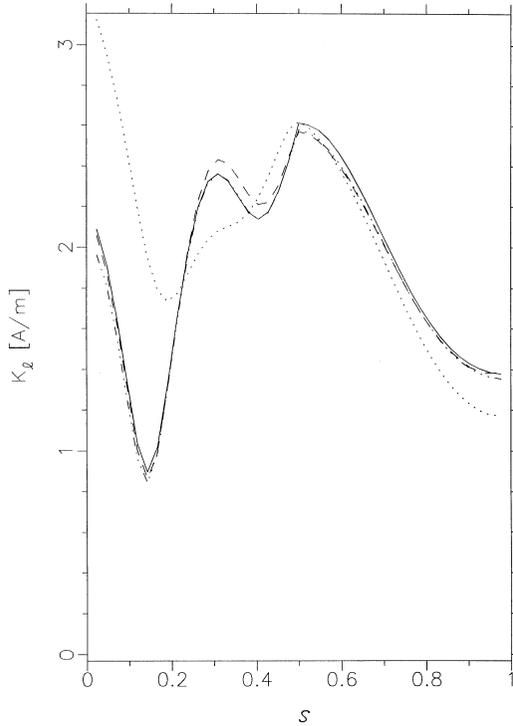
**Figure 10.** Magnitude of  $K_\ell$  on a half-buried metallic sphere with the parameters:  $\epsilon_1 = 10.0$ ,  $\epsilon_2 = 1.0$ ,  $\theta^i = 0.0^\circ$ ,  $k_0a = 1.035$ . EFIE: ....., MFIE: —, CFT: - · · ·, CHIEF: - - - .
