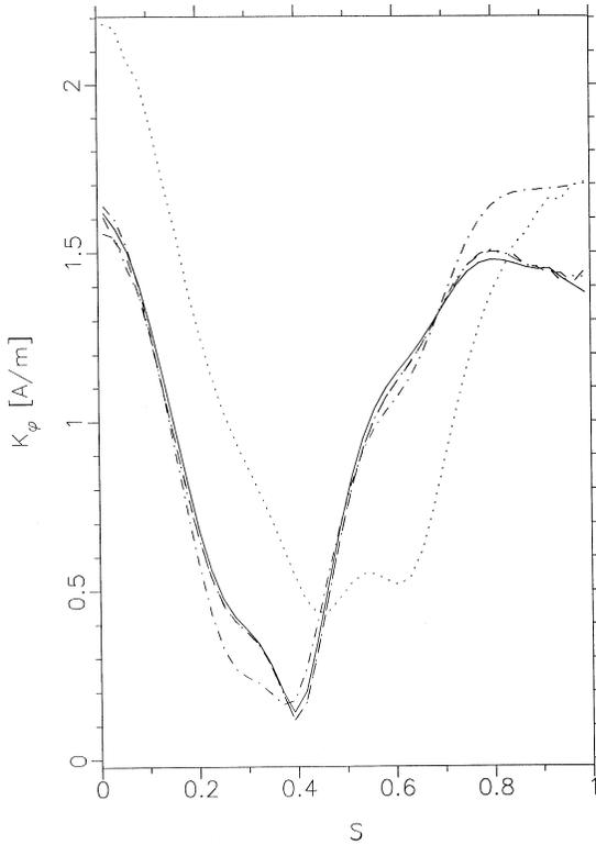
**Figure 6.** Magnitude of  $K_\varphi$  on a metallic sphere present in the upper space with the parameters:  $\epsilon_1 = 10.0$ ,  $\epsilon_2 = 1.0$ ,  $\theta^i = 0.0^\circ$ ,  $k_2a = 2.744$  and  $d = 0.2\lambda_o$ . EFIE: ....., MFIE: - · - ·, CFIE: —, CFT: - · · ·, CHIEF: - - - - .
