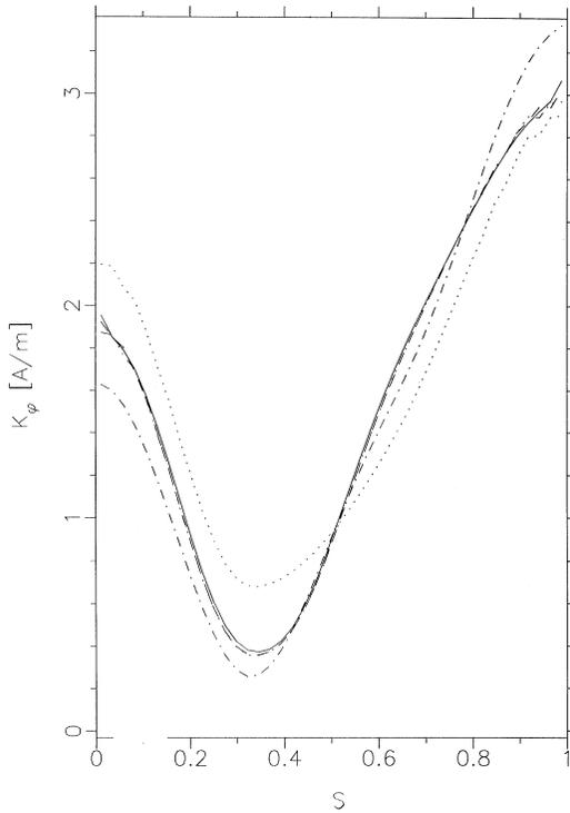
**Figure 8.** Magnitude of  $K_\varphi$  on a metallic sphere present in the lower space with the parameters:  $\epsilon_1 = 10.0$ ,  $\epsilon_2 = 1.0$ ,  $\theta^i = 0.0^\circ$ ,  $k_1 a = 2.744$  and  $d = -0.4\lambda_o$ . EFIE: ....., MFIE: - · - ·, CFIE: —, CFT: - · · ·, CHIEF: - - - .
