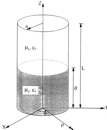
**Figure 17.** Partially filled circular cylindrical cavity.
