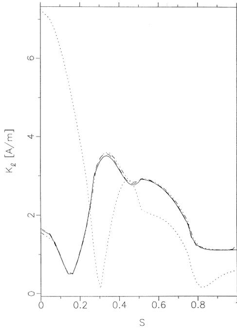
**Figure 15.** Magnitude of  $K_\ell$  on a half-buried metallic pillbox with the parameters:  $\epsilon_1 = 10.0$ ,  $\epsilon_2 = 1.0$ ,  $\theta^i = 0.0^\circ$ ,  $L/a = 2.0$  and  $k_o a = 0.9147$ . EFIE: ....., MFIE: —, CFT: - · · ·, CHIEF: - - - .
