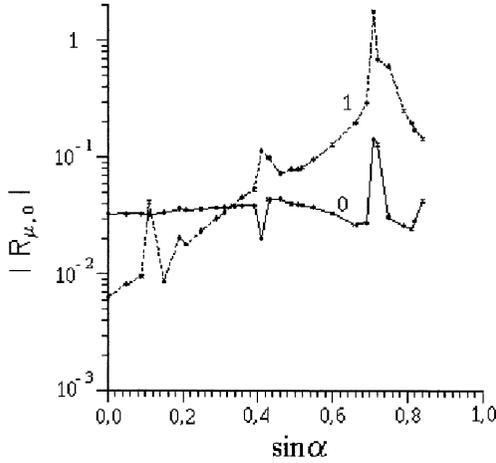
**Figure 5.** The dependence of the absolute value  $|R_{\mu,0}|$  of the Bloch reflection coefficient on the sine of the incidence angle,  $\sin \alpha$ , for modes  $\mu = 0, \pm 1$  and under conditions  $\epsilon = 1.50 + i0.20$ ,  $h/\lambda = 0.75$ ,  $\kappa = \lambda/\Lambda = 0.3$ .
