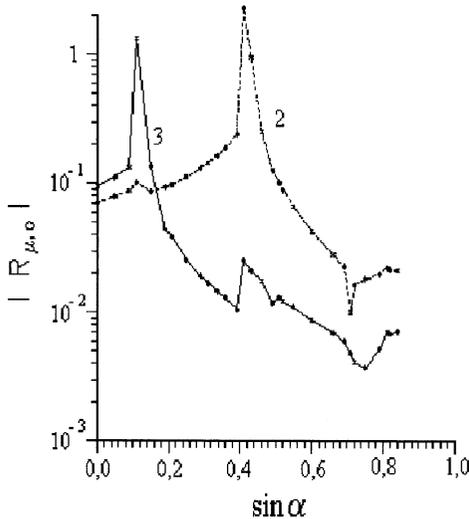
**Figure 6.** The dependence of the absolute value  $|R_{\mu,0}|$  of the Bloch reflection coefficient on the sine of the incidence angle,  $\sin \alpha$ , for modes  $\mu = \pm 2, \pm 3$  and under conditions  $\epsilon = 1.50 + i0.20$ ,  $h/\lambda = 0.75$ ,  $\kappa = \lambda/\Lambda = 0.3$ .
