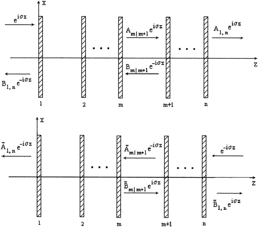
**Figure 1.** A three-dimensional medium presented as a stack of  $n$  layers with splits between them. In the top and bottom pictures the wave be incident upon the 1 st and the  $n$ 's layer of the stack, respectively.
