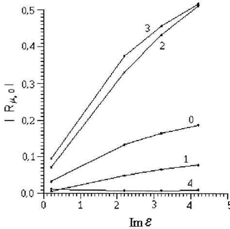
**Figure 3.** The dependence of the absolute value  $|R_{\mu,0}|$  of the Bloch reflection coefficient on the imaginary part  $\Im\epsilon$  of the lower half-space dielectric permittivity for modes  $\mu = 0, \pm 1, \pm 2, \pm 3, \pm 4$  and under conditions  $\Re\epsilon = 1.50$ ,  $\alpha = 0$ ,  $h/\lambda = 0.75$ ,  $\kappa = \lambda/\Lambda = 0.3$ .
