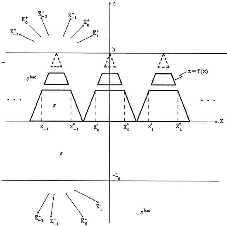
**Figure 2.** A periodic one-dimensional interface of two dielectric half-spaces with the dielectric permittivities  $\epsilon^{bac}$  (upper half-space) and  $\epsilon$  (lower half-space). An auxiliary truncated interface is presented in the form of a thin slice separated by a split from the rest truncated interface. The wave vectors of upgoing reflected and downcoming transmitted Bloch waves are depicted.
