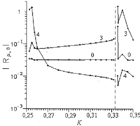
**Figure 4.** The dependence of the absolute value  $|R_{\mu,0}|$  of the Bloch reflection coefficient on the parameter  $\kappa = \lambda/\Lambda$  for modes  $\mu = 0, \pm 3, \pm 4$  and under conditions  $\epsilon = 1.50 + i0.20$ ,  $\alpha = 0$ ,  $h/\lambda = 0.75$ .
