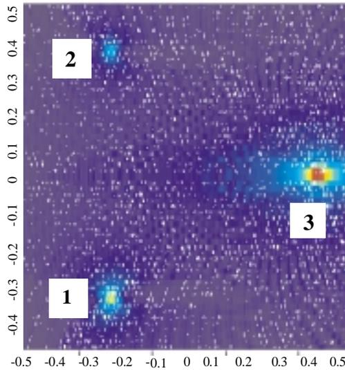
**Figure 4.2**  $E_\theta$  based image of the three scatterers.
