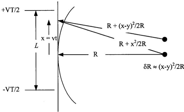
**Figure 2.2** Geometry for generating a synthetic aperture.
