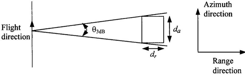
**Figure 2.1.** Side looking radar beam and resolution.
