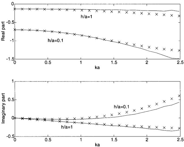
**Figure 9.** Real and imaginary parts of the normalized electric field  $E\epsilon_0 a^3 \exp(jkh)/p$  as functions of  $ka$ . Electric dipoles are orthogonal to the array plane. Exact (solid lines) and approximate ( $\times$ ) results.
