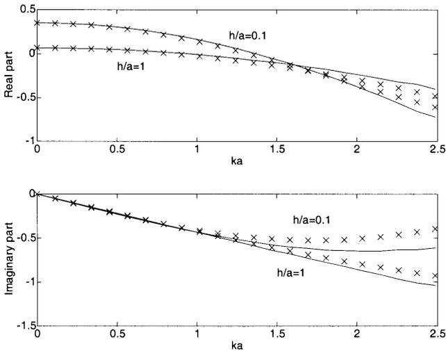
**Figure 7.** Real and imaginary parts of the normalized electric field  $E\varepsilon_0 a^3 \exp(jkh)/p$  as functions of  $ka$ . Electric dipoles are parallel to the array plane. Exact (solid lines) and approximate ( $\times$ ) results.
