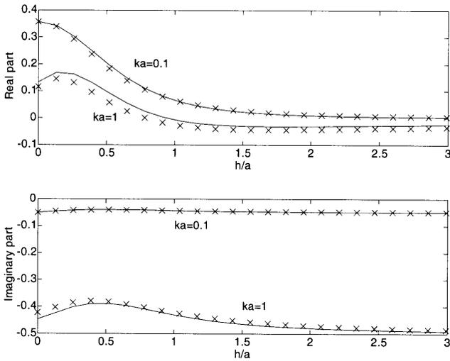
**Figure 4.** Real and imaginary parts of the normalized electric field  $E\varepsilon_0 a^3 \exp(jkh)/p$  as functions of  $h/a$ . Electric dipoles are parallel to the array plane. Exact (solid lines) and approximate ( $\times$ ) results.
