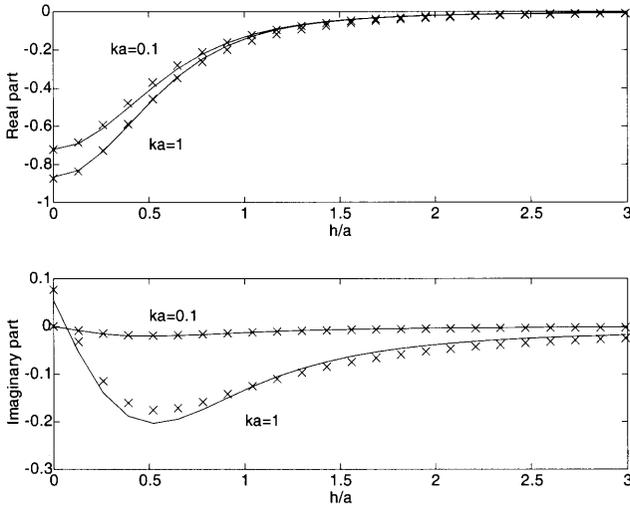
**Figure 6.** Real and imaginary parts of the normalized electric field  $E\varepsilon_0 a^3 \exp(jkh)/p$  as functions of  $h/a$ . Electric dipoles are orthogonal to the array plane. Exact (solid lines) and approximate ( $\times$ ) results.
