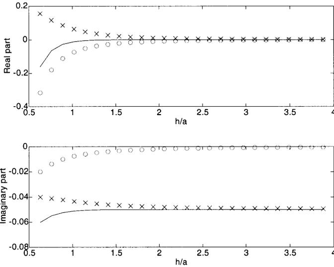
**Figure 10.** Real and imaginary parts of the normalized electric field  $E\varepsilon_0 a^3 \exp(jkh)/p$  as functions of  $h/a$  for  $ka = 0.1$ . Dipoles are parallel to the array plane. The field of the sheet with a hole ( $\times$ ), the field of the central dipole ( $\circ$ ) and their sum (solid lines).
