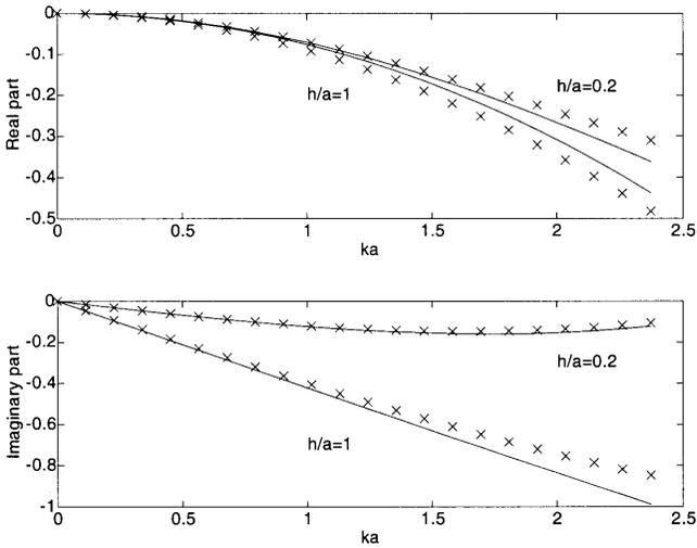
**Figure 8.** Real and imaginary parts of the normalized magnetic field  $H\eta\epsilon_0 a^3 \exp(jkh)/p$  as functions of  $ka$ . Electric dipoles are parallel to the array plane. Exact (solid lines) and approximate ( $\times$ ) results.
