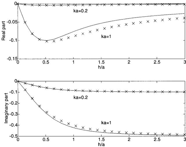
**Figure 5.** Real and imaginary parts of the normalized magnetic field  $H\eta\varepsilon_0 a^3 \exp(jkh)/p$  as functions of  $h/a$ . Electric dipoles are parallel to the array plane. Exact (solid lines) and approximate ( $\times$ ) results.
