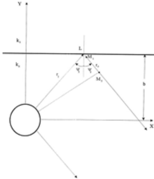
**Figure 3.** Ray diagram of scattered fields from buried cylinder for below the dielectric interface.
