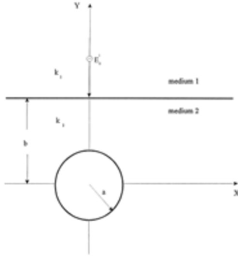
**Figure 1.** A perfectly conducting circular cylinder deeply buried in a dielectric half-space.
