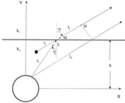
**Figure 2.** Ray diagram of scattered fields from buried cylinder for above the dielectric interface.
