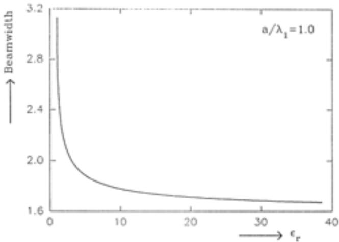
**Figure 5.b** The effect of relative dielectric constant  $\epsilon_r$  on the beamwidth.
