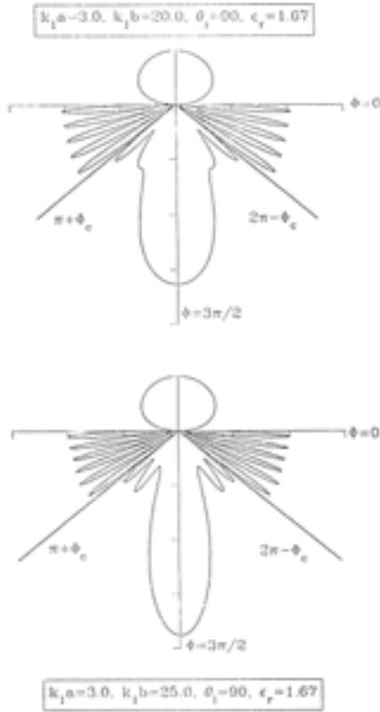
**Figure 4.** The normalized field pattern of buried cylinder.
