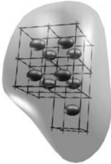
**Figure 1.** Homogenization of a photonic crystal made of ellipsoidal scatterers. The grid of dotted lines defines a virtual “scaffolding”  $\Omega_\eta$  of the whole obstacle  $\Omega_f$ . For the sake of simplicity, we give an example with  $\eta$  near from 1, i.e., with rather big scatterers and in a small number (here 9). The reader has to imagine the same body ( $\Omega_f$ ) filled with a great number of scatterers (on the order of 1000) of small size ( $\eta$  near from 0).
