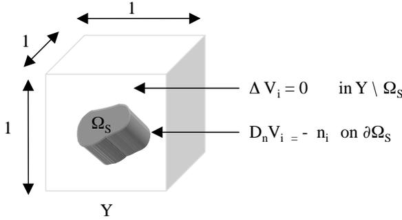
**Figure 9.** Description of the annex problem in the metallic case. One has to be careful if the scatterer touch the boundary of the unit cell: when some scatterers are stuck together to form a set of parallel rods, there are numerical inaccuracies.
