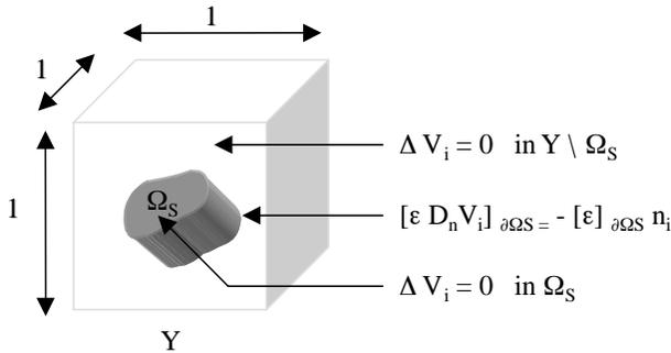
**Figure 8.** Description of the annex problem in the dielectric case. The scatterer can possibly touch the boundary of the elementary cell, which allows us studying dielectric structures made for example of parallel rods (Fig. 2).
