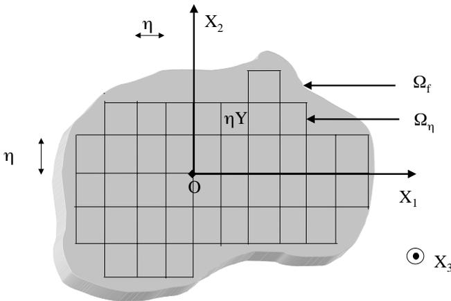
**Figure 5.** The process of homogenization consists in a periodic arrangement of rescaled unit cells, forming a succession of “scaffoldings”  $\Omega_\eta$  entirely enclosed in the diffracting object  $\Omega_f$ .
