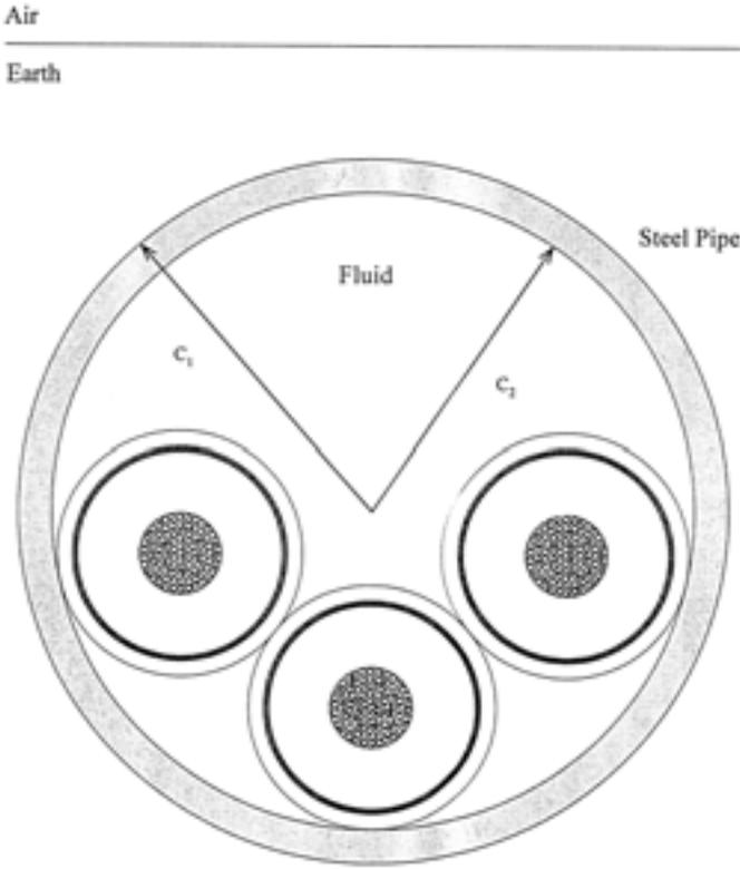
**Figure 1.** Cross-section of an underground three-phase pipe-type cable.
