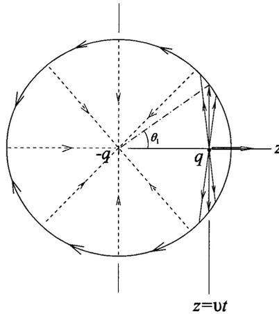
**Figure 2.** Fields of charge  $q$  moving with velocity  $v$ , and  $-q$  left at origin.
