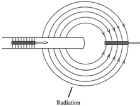
**Figure 8.** Beam exiting an open-ended pipe.
