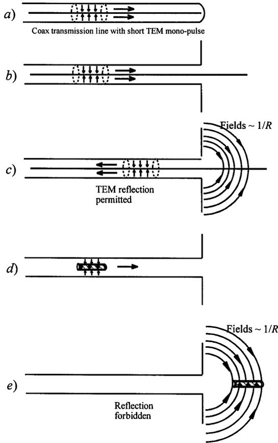
**Figure 10.** Beam radiation as extended transmission line fields.
