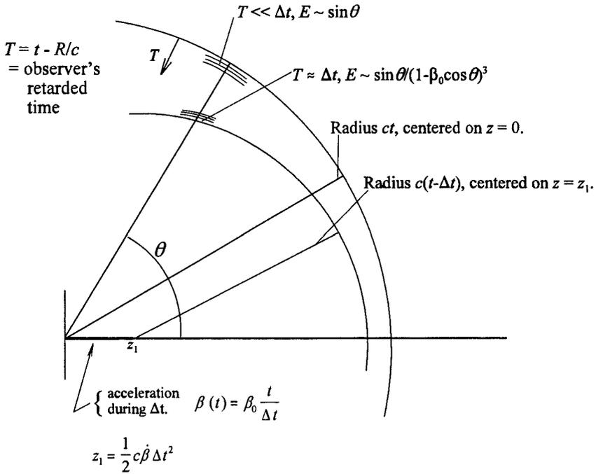
Figure 4. Field of a charge undergoing finite constant acceleration.
