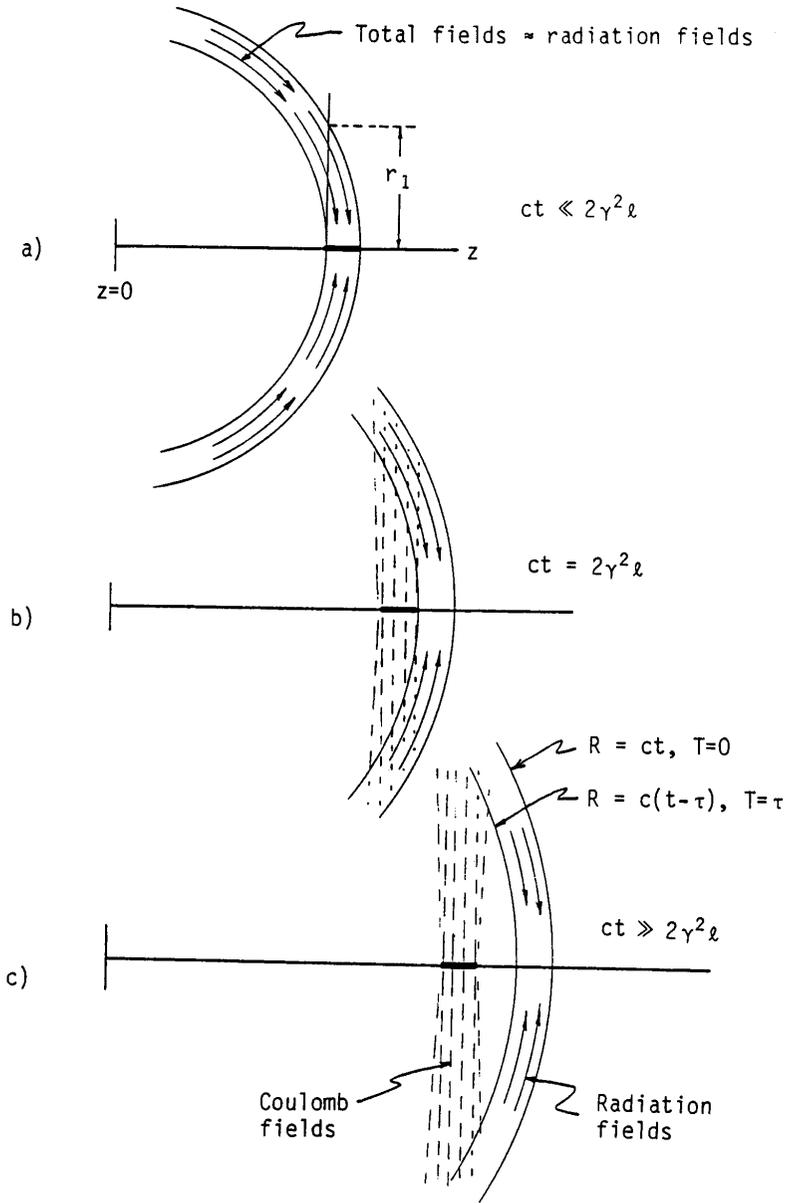
Figure 6. Developing field structure of a relativistic beam.
