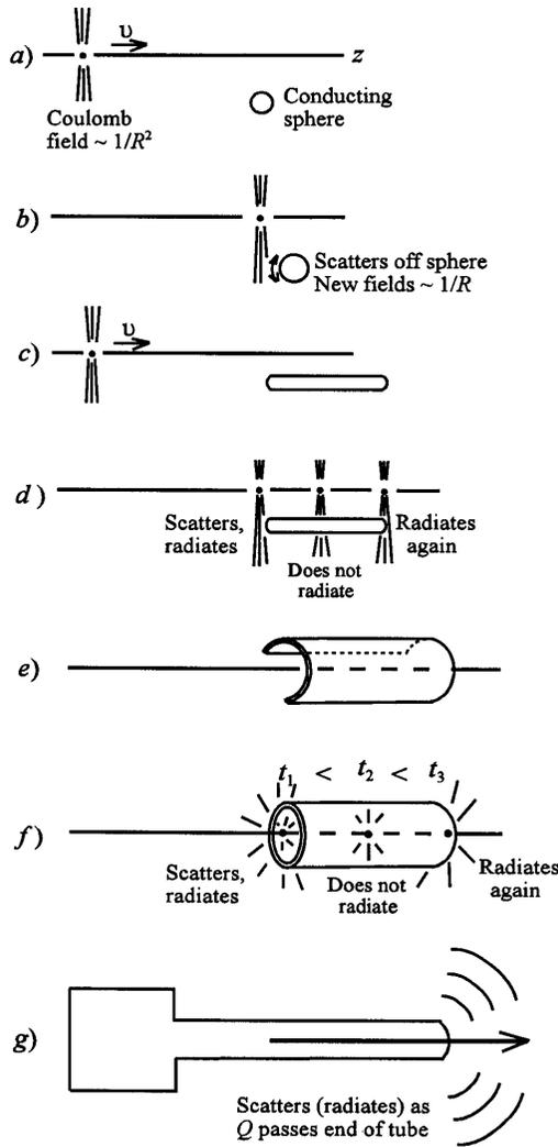
**Figure 9.** Showing how radiation of a beam exiting an open-ended pipe is equivalent to field scattering off a conductor.
