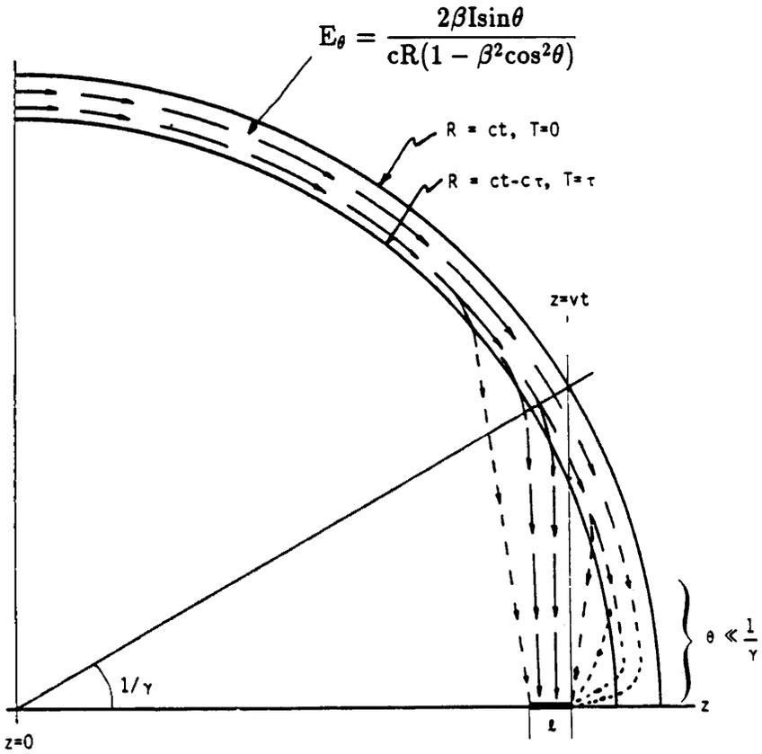
**Figure 7.** Field lines when  $ct \gg 2\gamma^2\ell$ . Field strength is indicated by length of line segment, not by line density.
