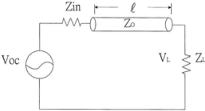
**Figure 8.** The equivalent circuit of the receiver.
