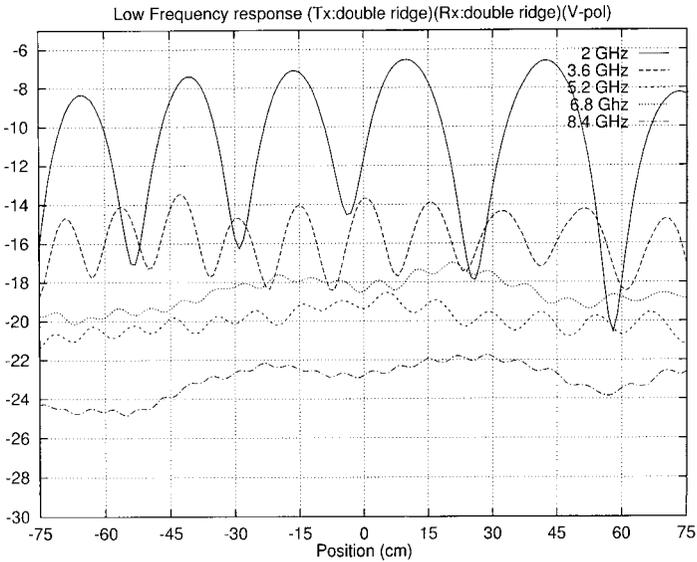
**Figure 4.** The amplitude distributions for different operating frequencies.
