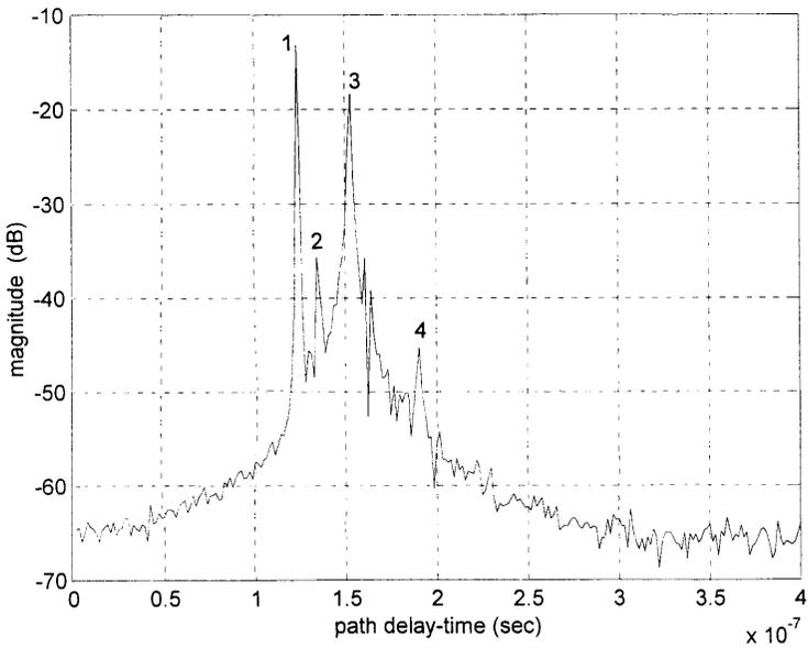
Figure 6. Range profiles with center frequency equal to 2.985 GHz .
