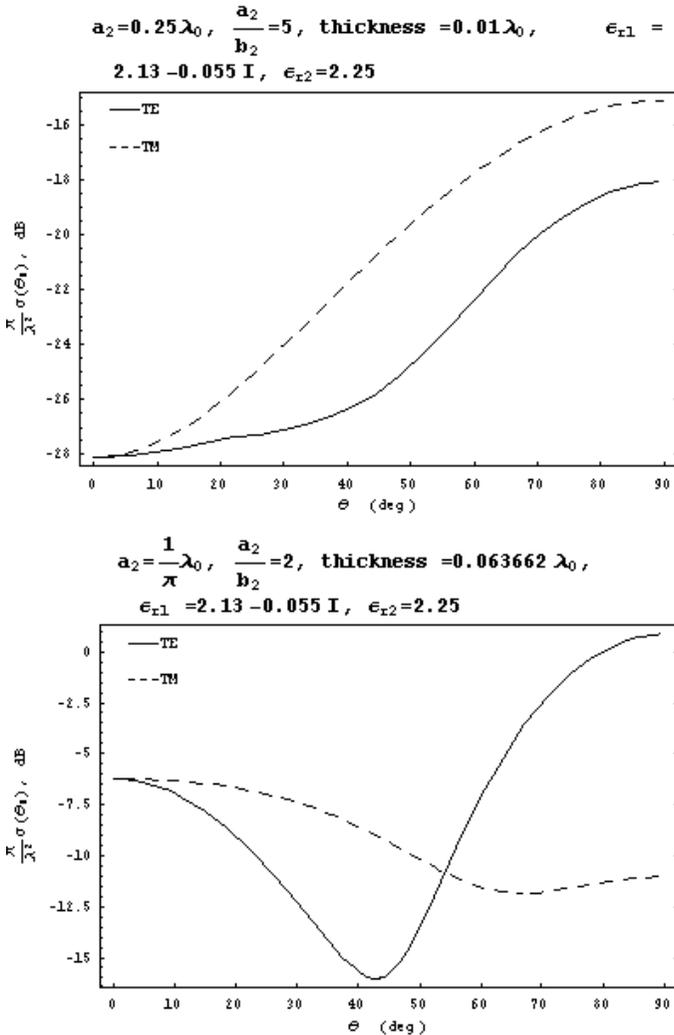
**Figure 5.** Backscatter cross-sections for coated dielectric spheroids with  $\epsilon_{r1} = 2.13 - 0.055i$ ,  $\epsilon_{r2} = 2.25$ , but different dimensions and coating thicknesses.
