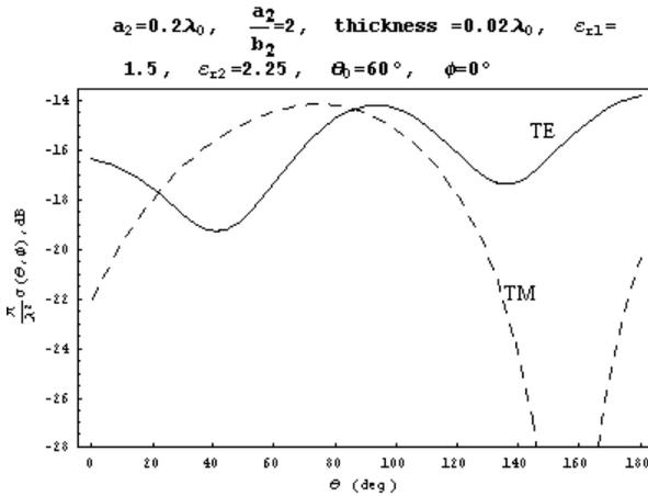
**Figure 6.** Bistatic cross-sections for a coated dielectric spheroid with  $a_2 = 0.2\lambda_0$ , axial ratio=2, coating thickness= $0.02\lambda_0$ ,  $\epsilon_{r1} = 1.5$  and  $\epsilon_{r2} = 2.25$ , at angles of incidence,  $20^\circ$ ,  $40^\circ$ ,  $60^\circ$ , and  $80^\circ$
