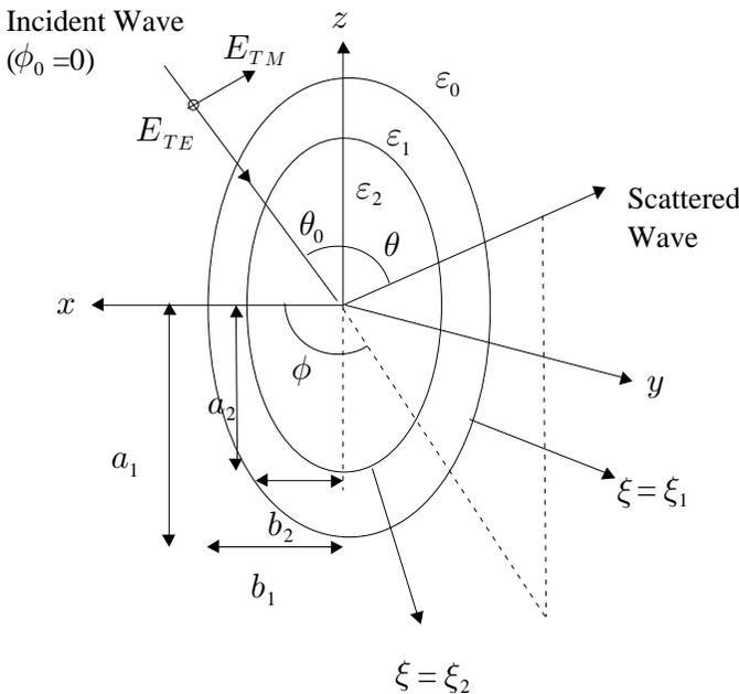
**Figure 2.** Scattering geometry for a coated dielectric spheroid.
