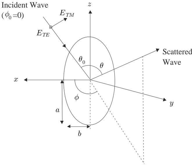
**Figure 1.** Scattering geometry for a prolate spheroid.
