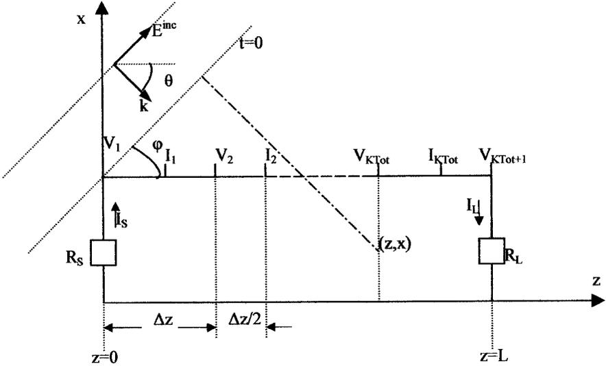
**Figure 3.** A uniform transmission line excited by an external electromagnetic wave.
