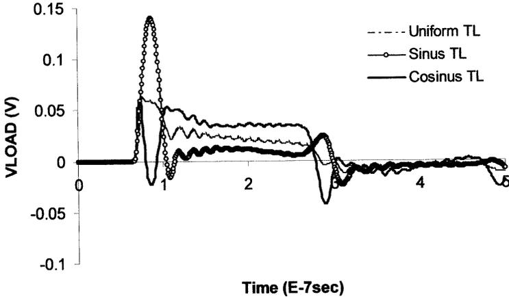
**Figure 11.** The comparison of far-end voltage of the transmission line configurations presented in comparison study 2.
