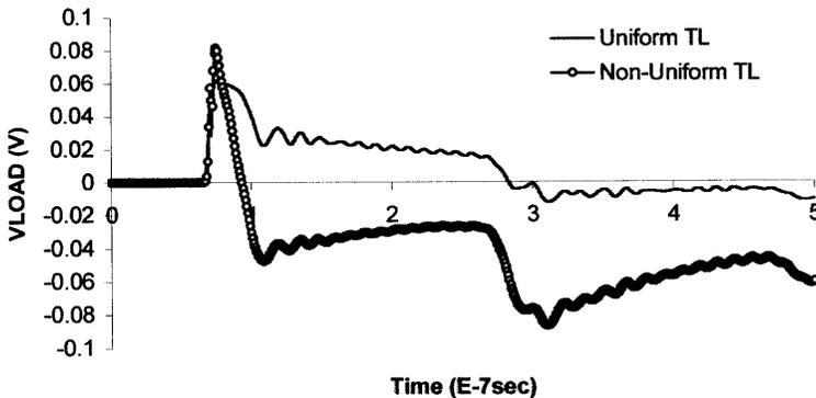
**Figure 7.** The induced voltage at the far-end of the uniform and non-uniform transmission line as described in Example 2.
