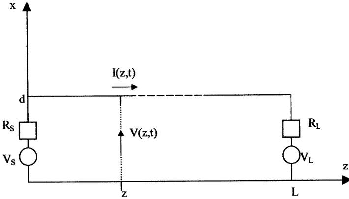
**Figure 1.** A uniform transmission line excited by lumped voltage sources.
