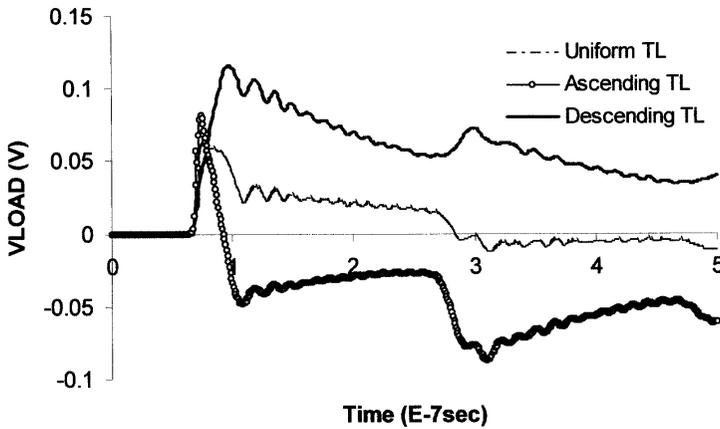
**Figure 9.** The comparison of far-end voltage of the transmission line configurations presented in comparison study 1.
