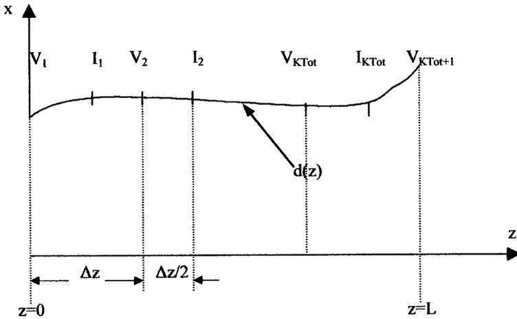
**Figure 4.** Arbitrary configuration of a non-uniform transmission line.
