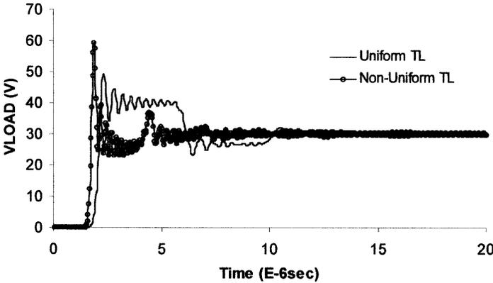
**Figure 5.** The induced voltage at the far-end of the uniform and non-uniform transmission line as described in Example 1.
