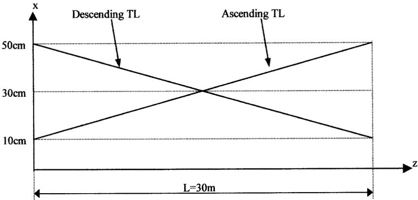
**Figure 8.** The configuration of non-uniform TL examined in comparison study 1.
