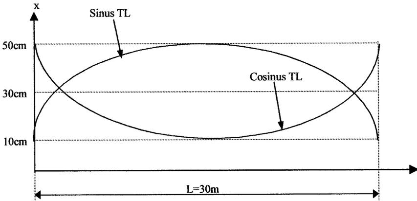
**Figure 10.** The configuration of non-uniform TL examined in comparison study 2.
