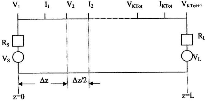
**Figure 2.** The spatial discretization of voltages and currents along the transmission line.
