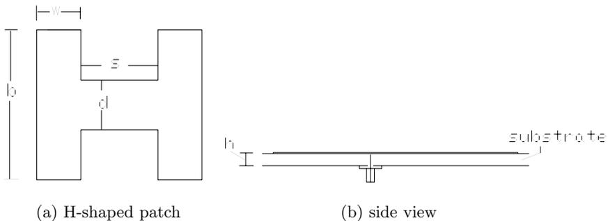
**Figure 1.** Configurations of the H-shaped patch antenna.
