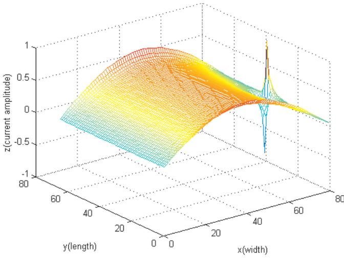
(a)  $J_x$  on ground plane
