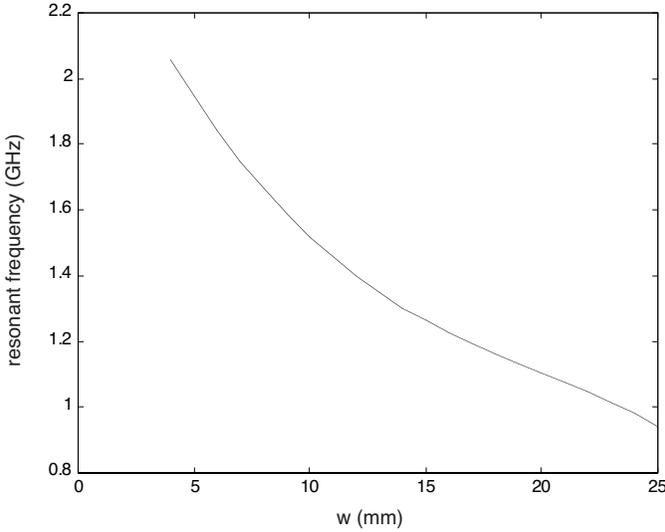
**Figure 5.** Variation of resonant frequency versus different values of the side strip length.
