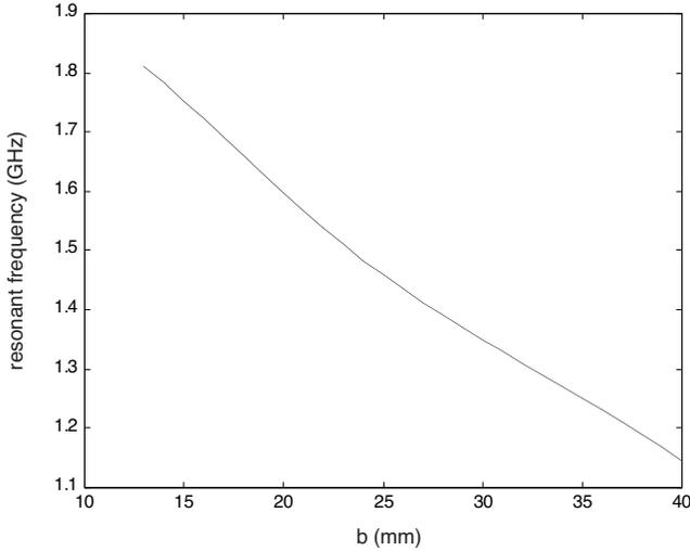
**Figure 6.** Variation of resonant frequency versus different values of the side strip width.
