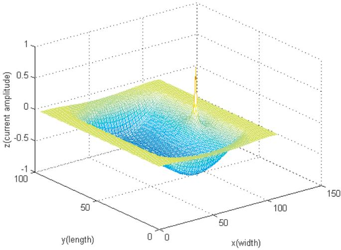
(c)  $J_x$  on ground plane
