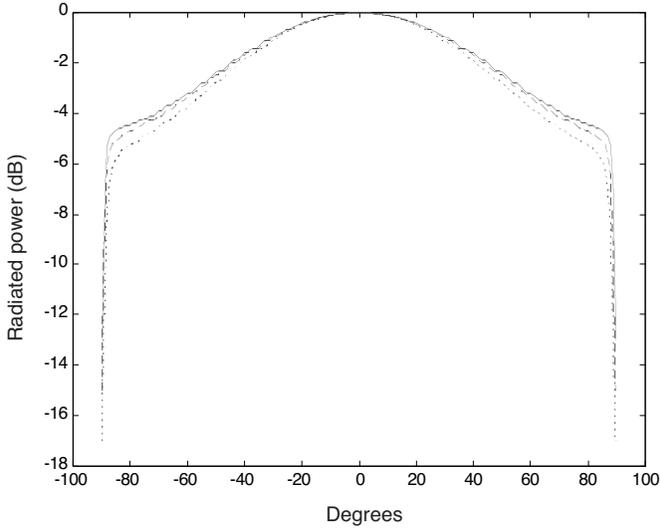
(a)  $E$ -plane pattern ( $\phi = 0^\circ$ )
