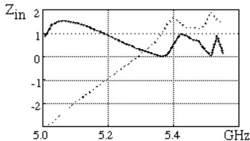
**Figure 7.** Real (solid curve) and imaginary (dotted curve) parts of the input impedance.
