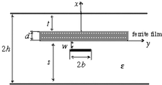
**Figure 2.** Cross-section of a strip-line MSW transducer.
