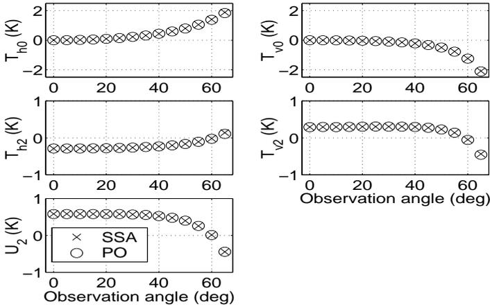
**Figure 2.**  $T_{h0}$ ,  $T_{v0}$ ,  $T_{h2}$ ,  $T_{v2}$ , and  $U_2$  for bi-sinusoidal surface with  $A = 1.501\lambda$ ,  $P_x = 50.001\lambda$ , and  $P_y = 100.001\lambda$  from twentieth order SSA and fourth order PO:  $0^\circ < \theta < 65^\circ$ .
