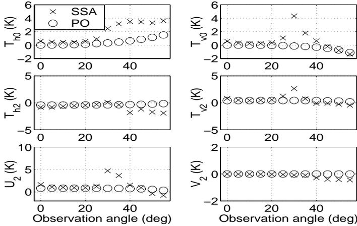
**Figure 7.**  $T_{h0}$ ,  $T_{v0}$ ,  $T_{h2}$ ,  $T_{v2}$ ,  $U_2$ , and  $V_2$  for bi-sinusoidal surface with  $A = 0.072\lambda$ ,  $P_x = 2.001\lambda$ , and  $P_y = 4.001\lambda$  from twentieth order SSA and fourth order PO:  $0^\circ < \theta < 55^\circ$ .
