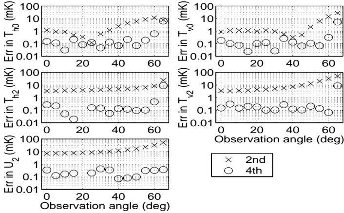
**Figure 3.** Error in  $T_{h0}$ ,  $T_{v0}$ ,  $T_{h2}$ ,  $T_{v2}$ , and  $U_2$  from second and fourth order SSA for bi-sinusoidal surface with  $A = 1.501\lambda$ ,  $P_x = 50.001\lambda$ , and  $P_y = 100.001\lambda$ :  $0^\circ < \theta < 65^\circ$ .
