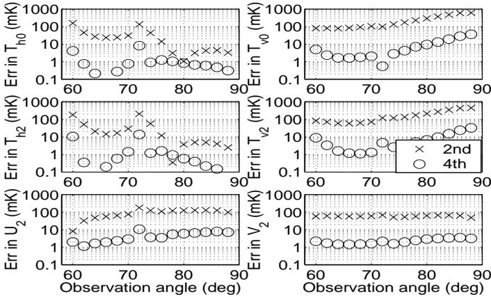
**Figure 10.** Error in  $T_{h0}$ ,  $T_{v0}$ ,  $T_{h2}$ ,  $T_{v2}$ ,  $U_2$ , and  $V_2$  from second and fourth order SSA for bi-sinusoidal surface with  $A = 0.072\lambda$ ,  $P_x = 2.001\lambda$ , and  $P_y = 4.001\lambda$ :  $60^\circ < \theta < 89^\circ$ .
