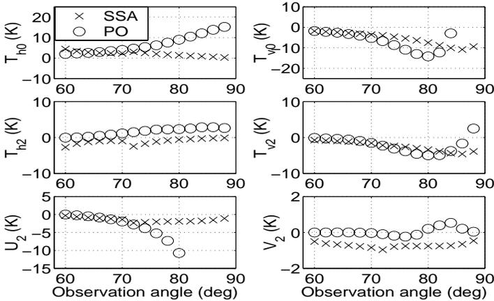
**Figure 9.**  $T_{h0}$ ,  $T_{v0}$ ,  $T_{h2}$ ,  $T_{v2}$ ,  $U_2$ , and  $V_2$  for bi-sinusoidal surface with  $A = 0.072\lambda$ ,  $P_x = 2.001\lambda$ , and  $P_y = 4.001\lambda$  from twentieth order SSA and fourth order PO:  $60^\circ < \theta < 89^\circ$ .
