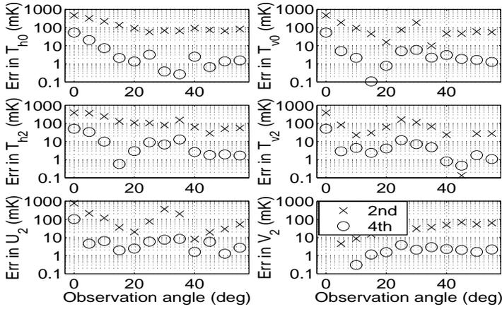
**Figure 8.** Error in  $T_{h0}$ ,  $T_{v0}$ ,  $T_{h2}$ ,  $T_{v2}$ ,  $U_2$ , and  $V_2$  from second and fourth order SSA for bi-sinusoidal surface with  $A = 0.072\lambda$ ,  $P_x = 2.001\lambda$ , and  $P_y = 4.001\lambda$ :  $0^\circ < \theta < 55^\circ$ .
