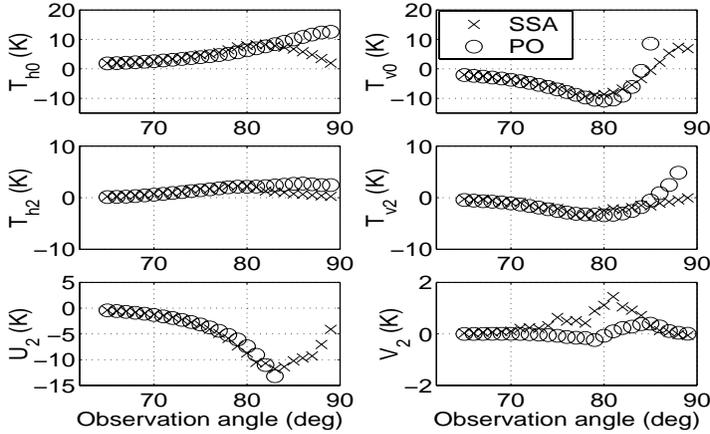
**Figure 4.**  $T_{h0}$ ,  $T_{v0}$ ,  $T_{h2}$ ,  $T_{v2}$ ,  $U_2$ , and  $V_2$  for bi-sinusoidal surface with  $A = 1.501\lambda$ ,  $P_x = 50.001\lambda$ , and  $P_y = 100.001\lambda$  from twentieth order SSA and fourth order PO:  $65^\circ < \theta < 89^\circ$ .
