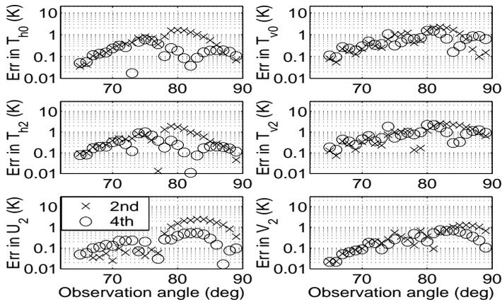
**Figure 5.** Error in  $T_{h0}$ ,  $T_{v0}$ ,  $T_{h2}$ ,  $T_{v2}$ ,  $U_2$ , and  $V_2$  from second and fourth order SSA for bi-sinusoidal surface with  $A = 1.501\lambda$ ,  $P_x = 50.001\lambda$ , and  $P_y = 100.001\lambda$ :  $65^\circ < \theta < 89^\circ$ .
