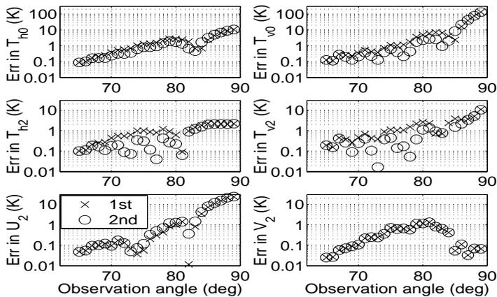
**Figure 6.** Error in  $T_{h0}$ ,  $T_{v0}$ ,  $T_{h2}$ ,  $T_{v2}$ ,  $U_2$ , and  $V_2$  from first and second order PO for bi-sinusoidal surface with  $A = 1.501\lambda$ ,  $P_x = 50.001\lambda$ , and  $P_y = 100.001\lambda$ :  $65^\circ < \theta < 89^\circ$ .
