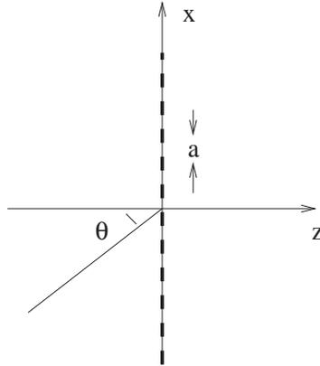
**Figure 1.** Planar dipole array, oblique plane wave incidence.
