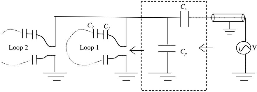
**Figure 7.** Circuit diagram of a RF coil in time-harmonic case.
