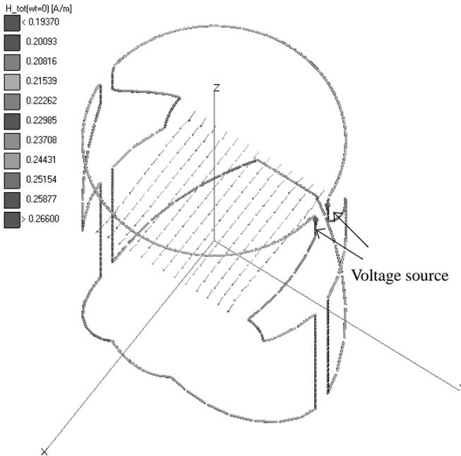
**Figure 10.** Time-harmonic solution for a side excited RF coil computed by GA/MoM code; and distribution of transverse magnetic field  $B_x$  in the  $z = 50$  mm plane.
