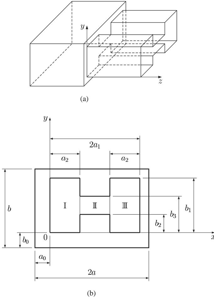
**Figure 2.** Empty-to-ridge waveguide discontinuity. (a) Configuration. (b) Discontinuity plane.
