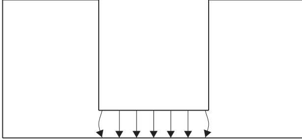
**Figure 7.** (Electric) field distribution of the ridge waveguide.
