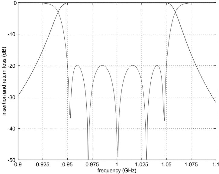
**Figure 5.** Computed response of the five-section 1-GHz filter.
