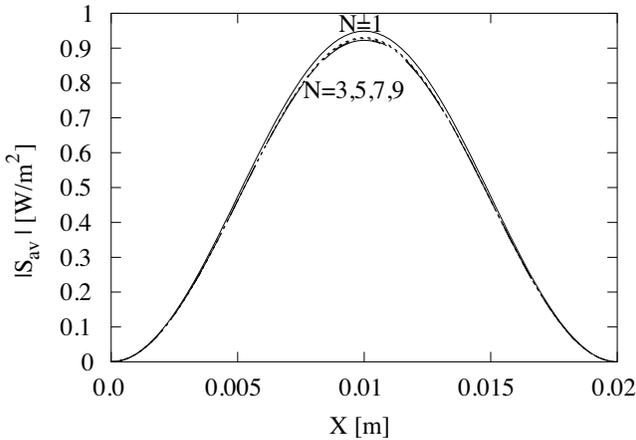
**Figure 3.** A solution of the output power density ( $|S_{av}|$ ) as a response to a  $TE_{10}$  input wave and a circular dielectric profile for  $N = 1, 3, 5, 7,$  and  $9$ , where  $a = b = 2$  cm,  $r_1 = 0.5$  mm,  $z = 20$  cm,  $\lambda = 3.75$  cm,  $y = b/2$ , and  $\epsilon_r = 2.25$ .
