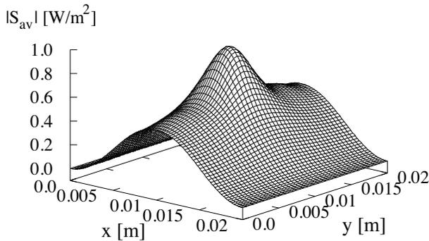
**Figure 6.** A solution of the output power density ( $|S_{av}|$ ) as a response to a  $TE_{10}$  input wave and a circular dielectric profile for where  $a = b = 2$  cm,  $r_1 = 0.5$  mm,  $z = 20$  cm,  $\lambda = 3.75$  cm, and  $\epsilon_r = 10$ .
