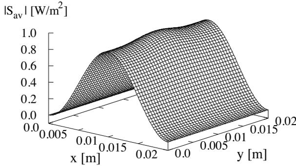
**Figure 4.** A solution of the output power density ( $|S_{av}|$ ) as a response to a  $TE_{10}$  input wave and a circular dielectric profile where  $a = b = 2$  cm,  $r_1 = 0.5$  mm,  $z = 20$  cm,  $\lambda = 3.75$  cm, and  $\epsilon_r = 2.25$ .
