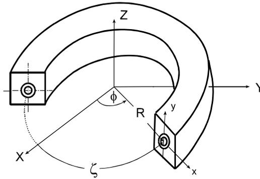
**Figure 1.** The curved coordinate system  $(x, y, \zeta)$ .
