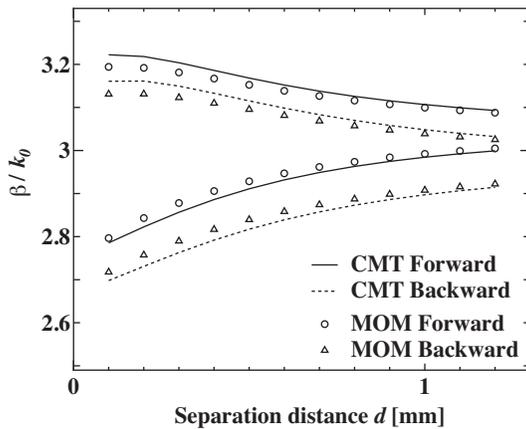
**Figure 5.** Forward and backward normalized propagation constants of two identical microstrip lines as functions of the separation distance  $d$ , where  $w_1 = w_2 = 0.254$  mm,  $h_1 = 0.254$  mm,  $\epsilon_r = 12.6$ ,  $f = 10$  GHz,  $\mu_0 H_i = 0.0275$  T and  $\mu_0 M_i = 0.275$  T. Note that CMT refers to the coupled-mode theory which presented here, and MOM refers to the Galerkin moment method.
