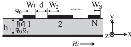
**Figure 2.** Cross section of  $N$  coupled microstrip lines on a Magnetized ferrite substrate.
