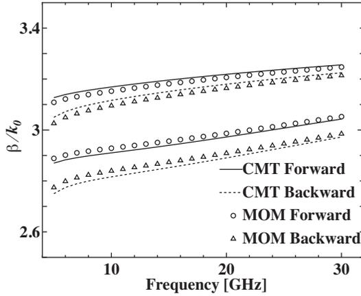
**Figure 4.** Forward and backward normalized propagation constants of two identical microstrip lines as functions of frequency, where  $w_1 = w_2 = 0.254$  mm,  $h_1 = 0.254$  mm,  $\epsilon_r = 12.6$ ,  $d = 0.5$  mm,  $\mu_0 H_i = 0.0275$  T, and  $\mu_0 M_i = 0.275$  T. Note that CMT refers to the coupled-mode theory which presented here, and MOM refers to the Galerkin moment method.
