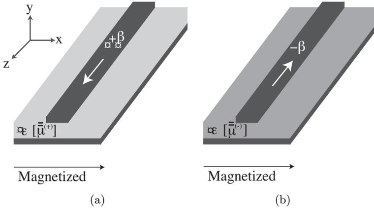
**Figure 1.** Two sets of guided-wave fields propagate in the ferrite. (a)The guided-wave  $(\mathbf{E}^{(+)}, \mathbf{H}^{(+)}, \mathbf{J}^{(+)})$  propagate in the  $+z$  direction, (b)The guided-wave  $(\mathbf{E}^{(-)}, \mathbf{H}^{(-)}, \mathbf{J}^{(-)})$  propagate in the  $-z$  direction.
