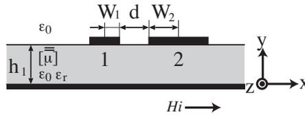
**Figure 3.** Cross section of two coupled microstrip lines on a magnetized ferrite substrate.
