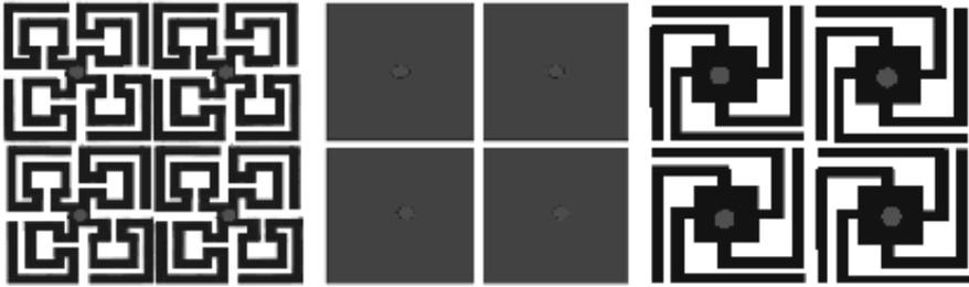
**Figure 3.** The three objects of comparison (top view): a grid of spiral-shaped elements with loops (left), a grid of patches (center), and a grid of spiral-shaped elements without loops (right).
