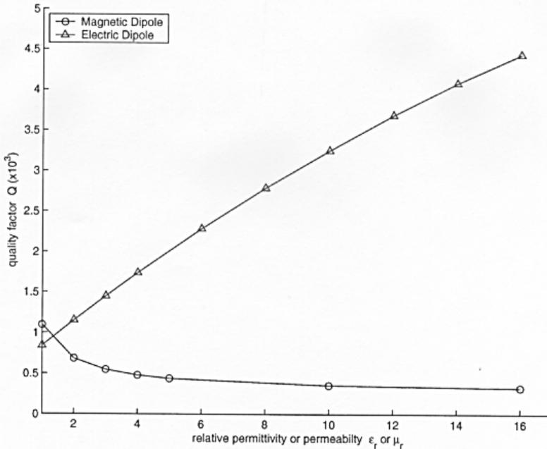
**Figure 4.** A modeled (HFSS) comparison of the effect of material loading on the free-space  $Q$  of a small magnetic and electric field antenna. An improvement in the  $Q$  of the small magnetic loop antenna is shown as a function of the relative permeability ( $\mu_r > 1$ ) of the material in the antenna sphere. A similar reduction is not observable with the equivalently sized electric dipole surrounded by a higher permittivity ( $\epsilon_r > 1$ ) material.
