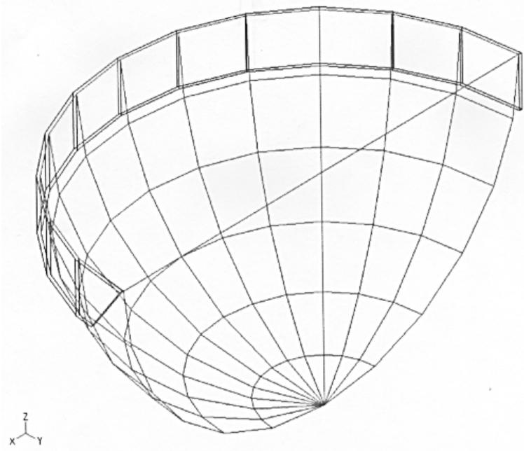
**Figure 2.** HFSS model of the experimental magnetic loop antenna. A symmetric  $H$ -plane and  $E$ -plane was used to simplify the geometry to help facilitate simulation convergence. The use of symmetry planes reduces the problem space to one quarter of the original size.
