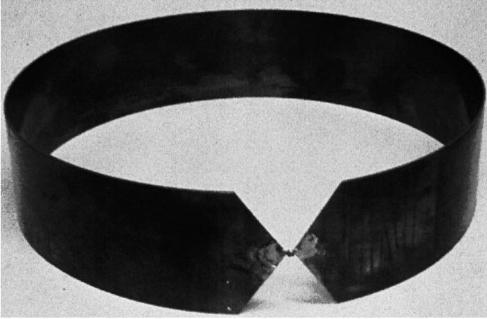
**Figure 1.** The experimental magnetic loop antenna used for the  $Q$  measurements above a “real ground” half-space. The low ESR capacitor used to tune the loop is shown in the foreground at the feed-point of the loop antenna.
