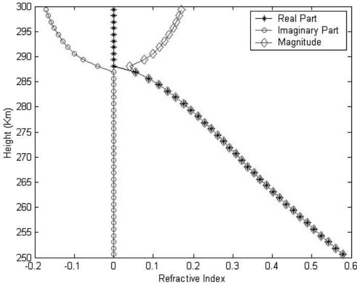
**Figure 1.** Refractive index around the reflection level.
