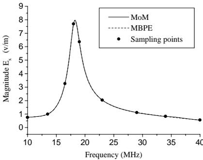
(a)  $E_{sca}^x$  component
