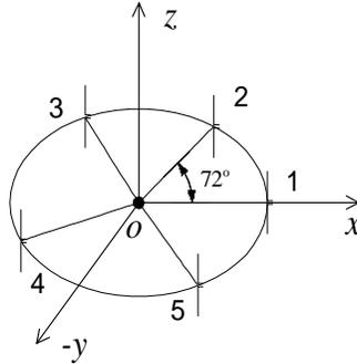
**Figure 6.** Five-element circular array for finding direction.
