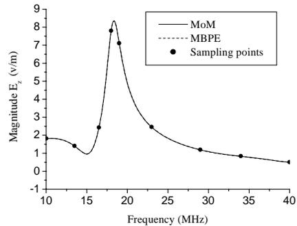
(b)  $E_{sca}^z$  component**Figure 11.** Frequency responses of the scattered near field magnitude.
