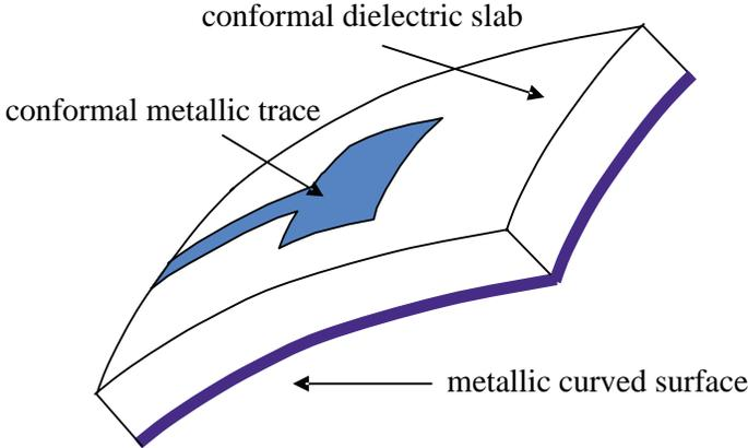
**Figure 1.** An example of an integrated conformal structure.
