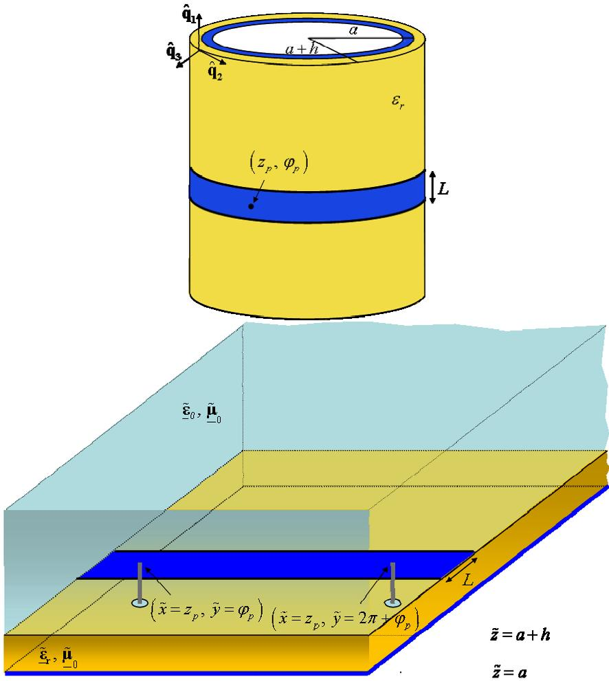
**Figure 4.** (a) Wrap-around cylindrical patch antenna. The geometrical and electrical parameters are:  $L = 80$  mm,  $h = 1.6$  mm,  $a = 20$  mm,  $z_p =$  upper patch edge position,  $\varphi_p = 0$ ,  $\epsilon_r = 4.2 + j0.02$ . (b) Isomorphic planar structure.
