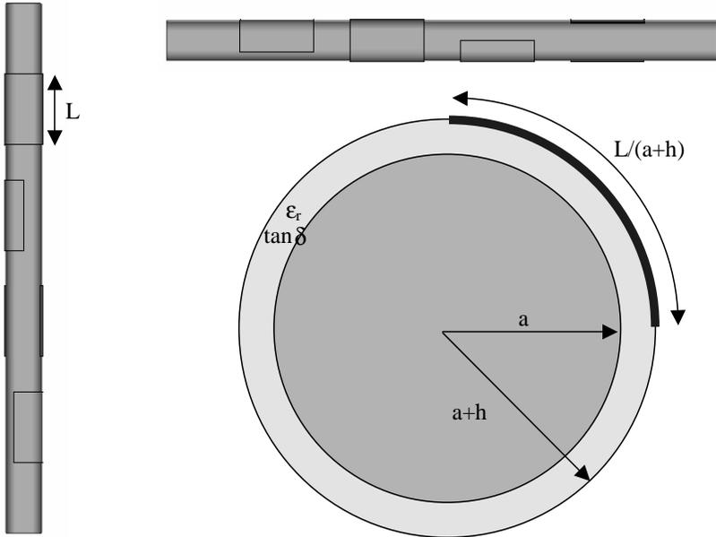
**Figure 6.** Geometry of an array of four patches on a cylindrical substrate with a cylindrical ground plane. The geometrical and electrical parameters of the structure are:  $L = 0.155$  m;  $a = 0.05$  m;  $h = 0.0016$ ;  $\epsilon_r = 1.15$ ;  $\tan \delta = 0.001$ .
