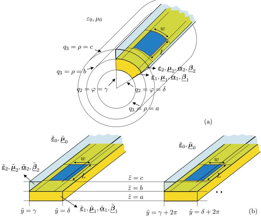
**Figure 3.** (a) Conformal metallic patch mounted on a cylindrical support and (b) its isomorphic geometry. The associated reference systems are:  $\hat{\mathbf{q}}_1 = \hat{\mathbf{z}}$ ,  $\hat{\mathbf{q}}_2 = \hat{\boldsymbol{\varphi}}$ ,  $\hat{\mathbf{q}}_3 = \hat{\boldsymbol{\rho}}$ ;  $h_1 = h_3 = 1$ ,  $h_2 = \rho$  for Fig. 3a and  $\hat{\mathbf{q}}_1 = \hat{\mathbf{x}}$ ,  $\hat{\mathbf{q}}_2 = \hat{\mathbf{y}}$ ,  $\hat{\mathbf{q}}_3 = \hat{\mathbf{z}}$  for Fig. 3b.
