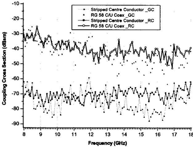
**Figure 6.** Comparison of coupling cross section between the RC and GC methodologies.
