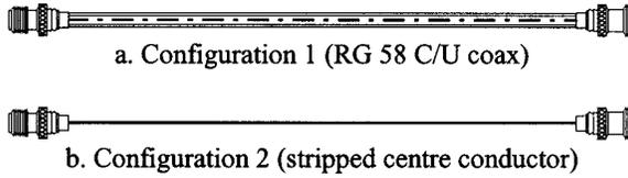
**Figure 2.** Two different cable configurations under test.
