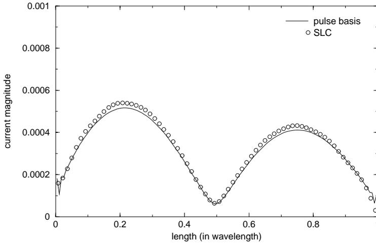
**Figure 3.** The normalized current magnitude: straight-wire scatterer.
