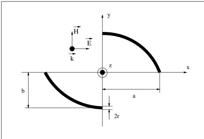
**Figure 4.** The thin-wire scatterer.
