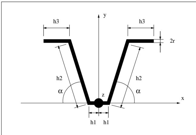
**Figure 7.** Geometry of the gull-shaped piecewise linear antenna.
