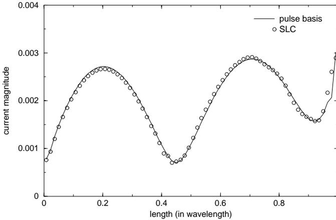
**Figure 6.** The normalized current magnitude: straight-wire antenna.
