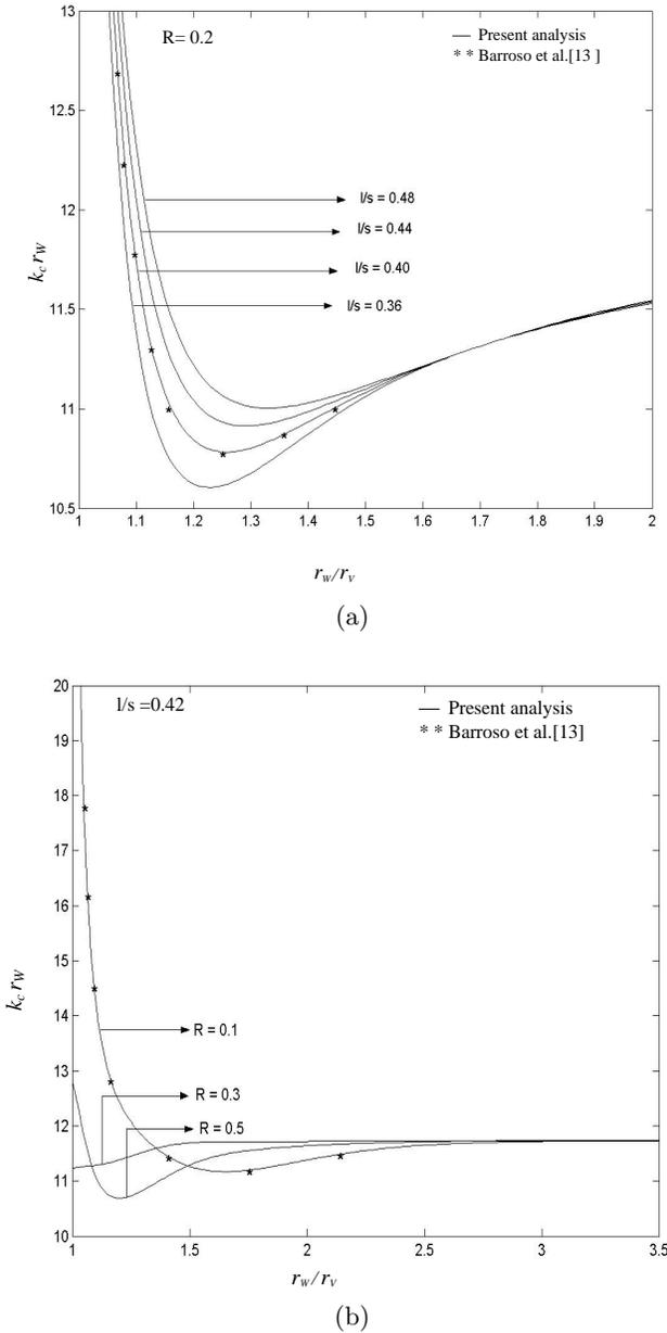
**Figure 3.** Variation of the eigenvalue of the typical waveguide mode  $TE_{6,2}$  with the ratio of the waveguide to ridge radii for configuration A, taking the slot width relative to the ridge periodicity (a) and the ridge depth relative to the outer ridge-edge radius (b) as the parameters.
